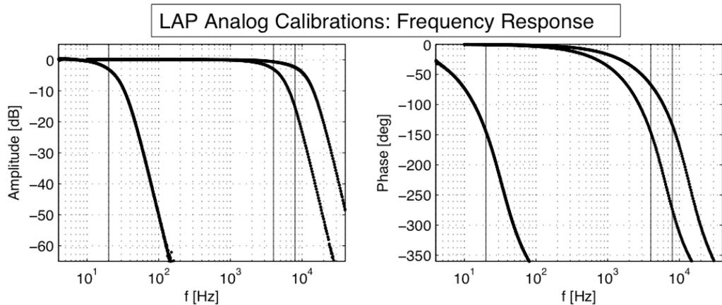
**Figure 2.** The frequency response of the LAP instrument, showing the rolloff of the anti-aliasing filters, as obtained during laboratory tests of the flight hardware. Data for P1 and P2 are plotted on top of each other: the probes are identical to the limit of this plot resolution.
