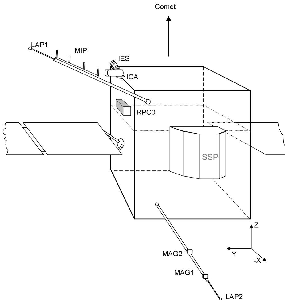
**Figure 1.** The mounting of the LAP sensors, LAP1 and LAP2, and other RPC units on the Rosetta spacecraft. RPC-0 is the common electronics box, also housing the LAP electronics boards. The direction of the s/c coordinate axes are indicated: the origin of the s/c coordinate system is at the centre of the  $-Z$  surface (bottom surface in this sketch). SSP is the Philae lander, not part of RPC. [From RD3]
