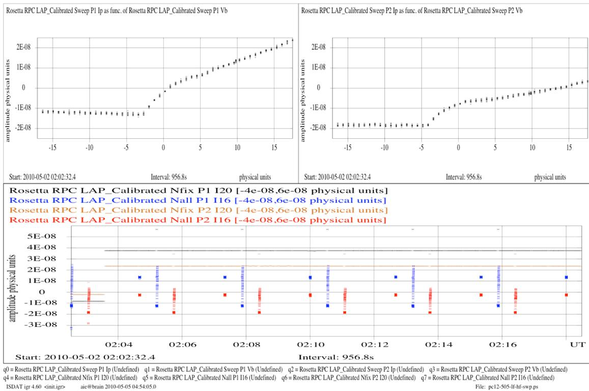
**Figure 3.** Data from the test of macro 0x505. Photoemission saturation currents: P1 13 nA, P2 18 nA (but note the vertical displacement of the P2 data, see text).
