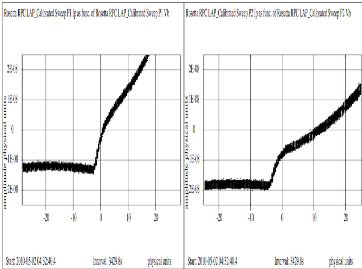
**Figure 5.** Data from macro 0x212 in RP10. Photoemission saturation currents: P1 13 nA, P2 18 nA (but note the vertical displacement of the P2 data, see text).
