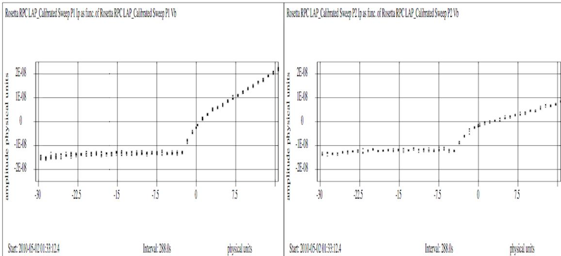
**Figure 4.** Data from the initial run of macro 0x212 in RP10. Photoemission saturation currents: P1 13 nA, P2 12 nA.
