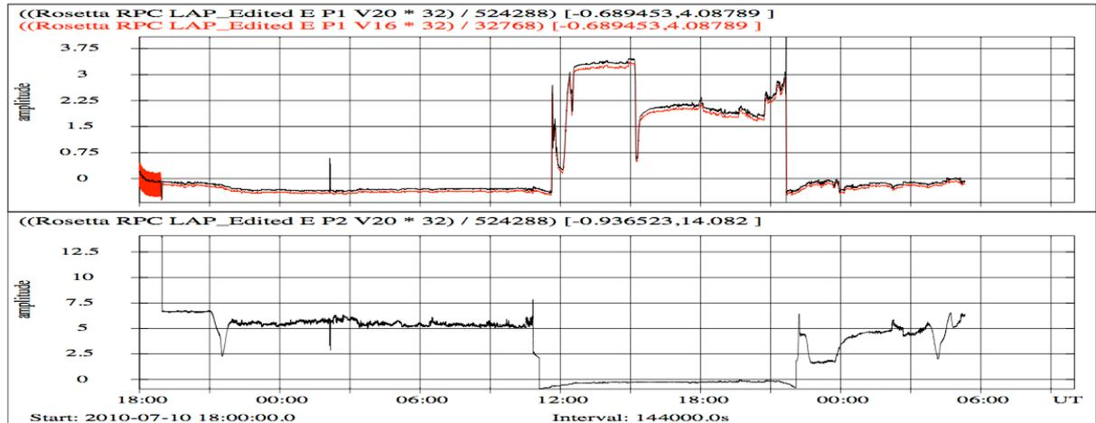
**Figure 9.** Probe 1 and 2 voltages (in volts) during block F. Red is 16-bit snapshots at 18.75 kHz sampling frequency, black 20-bit voltages at 57.8 Hz.
