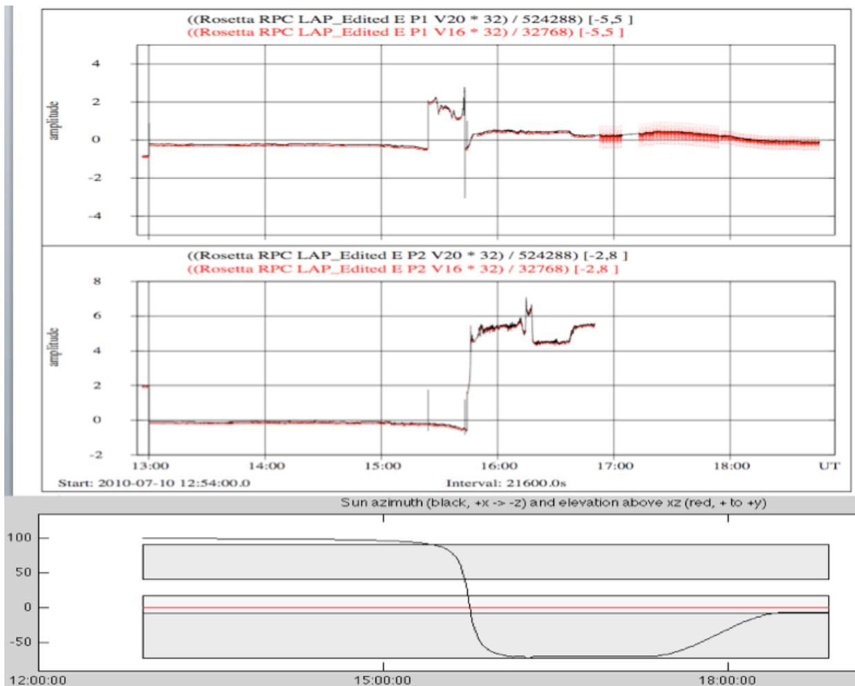
**Figure 7.** Probe 1 and 2 voltages (in volts) during a period of solar aspect angle around 100 degrees. In the two upper plots, red indicates 16-bit snapshots at 18.75 kHz sampling frequency, while black is 20-bit voltages at 57.8 Hz.
