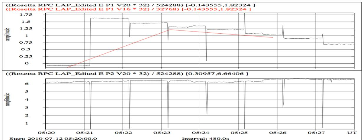
**Figure 10.** Probe 1 and 2 voltages (in volts) during bias current stepping on P1 (block G). Red is 16-bit snapshots at 18.75 kHz sampling frequency, black 20-bit voltages at 57.8 Hz.
