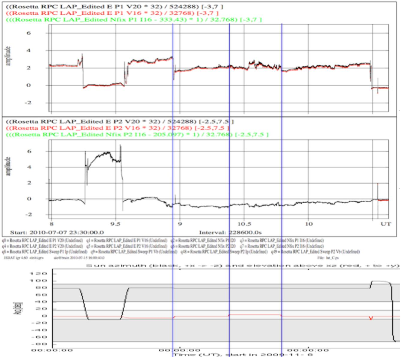
**Figure 6.** LAP probe voltages (in volts) for P1 (upper panel) and P2 (centre panel) during the approach to Lutetia, with spacecraft pointing as in Figure 2 (lower panel). Blue vertical lines indicate some of the times when the pointing of the s/c Y axis (red line in lower plot) changes. In the top plot, red is 16-bit snapshots at 18.75 kHz sampling frequency, black 20-bit voltages at 57.8 Hz.
