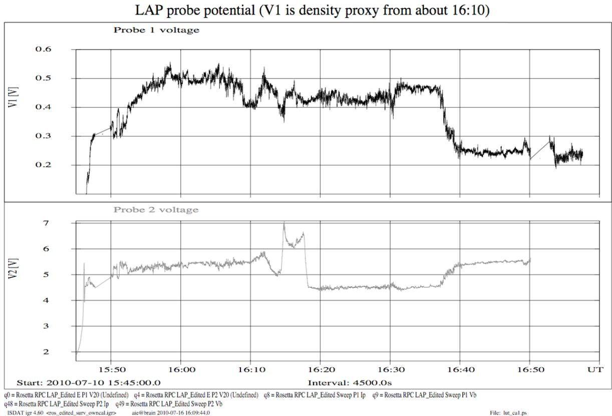
**Figure 8.** Probe 1 and 2 voltages (in volts, sampled at 57.8 Hz) around closest approach.
