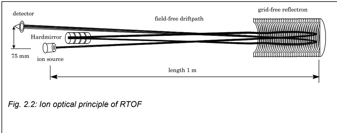
Fig. 2.2: Ion optical principle of RTOF
