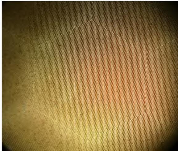
Figure 26: Picture of an MCP with the hexagonal structure due to fabrication fashion. The structure causes a modulation in the individual pixel gain of 24 pixels.
