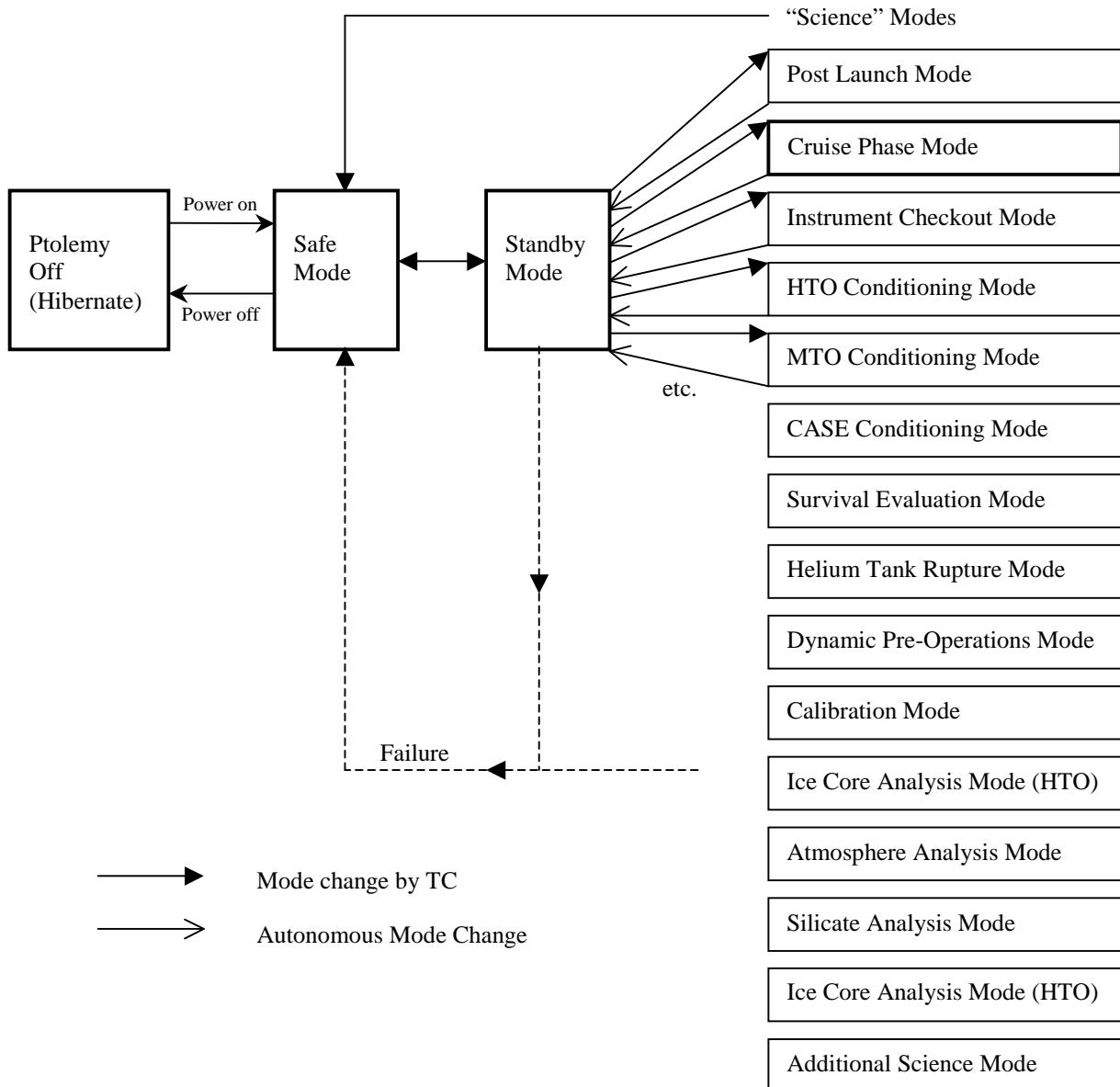
*Figure 1. Schematic of the Ptolemy operational modes and permitted mode transitions.*
