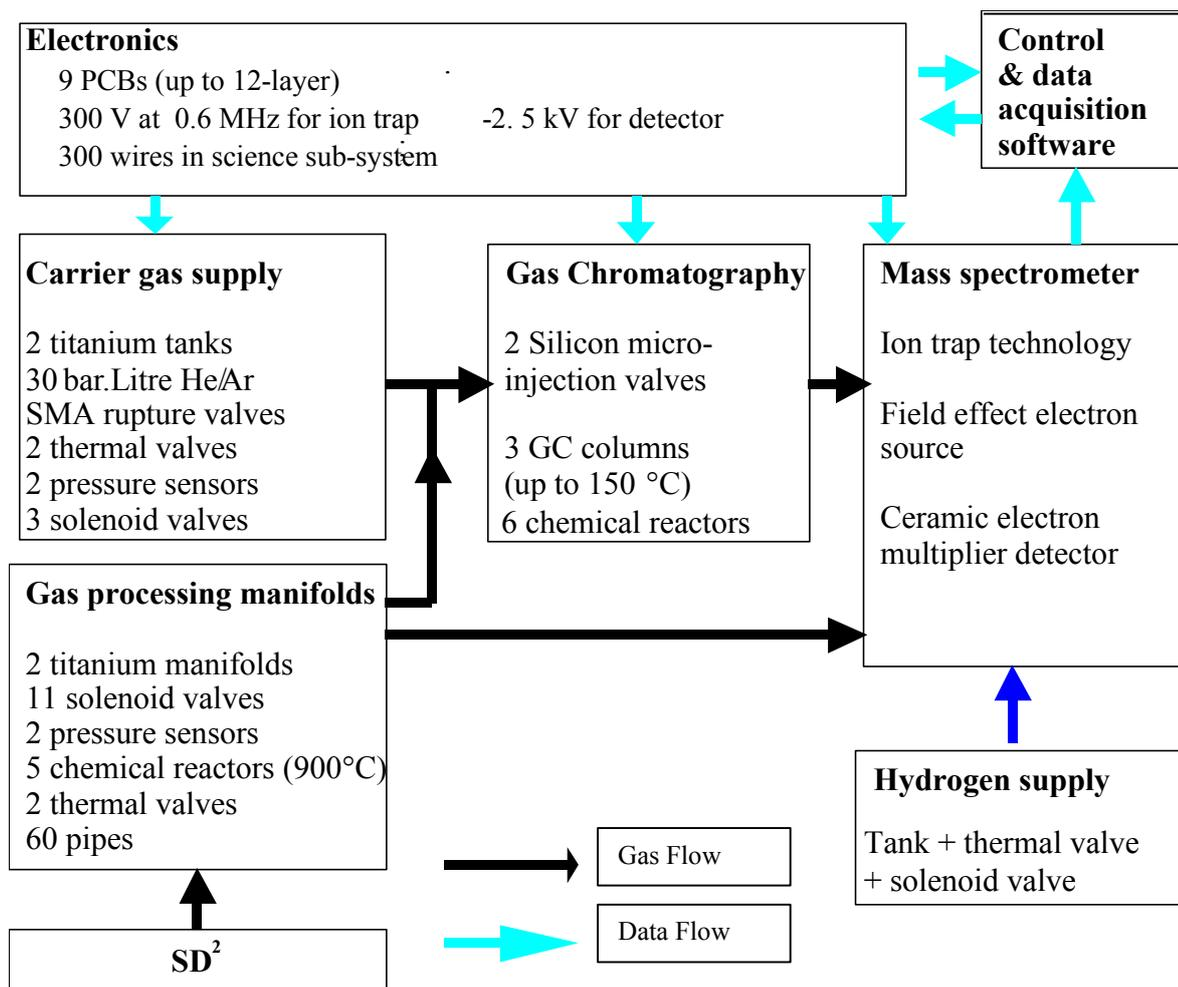
Figure 1: Schematic representation of the components required to process samples within Ptolemy.
