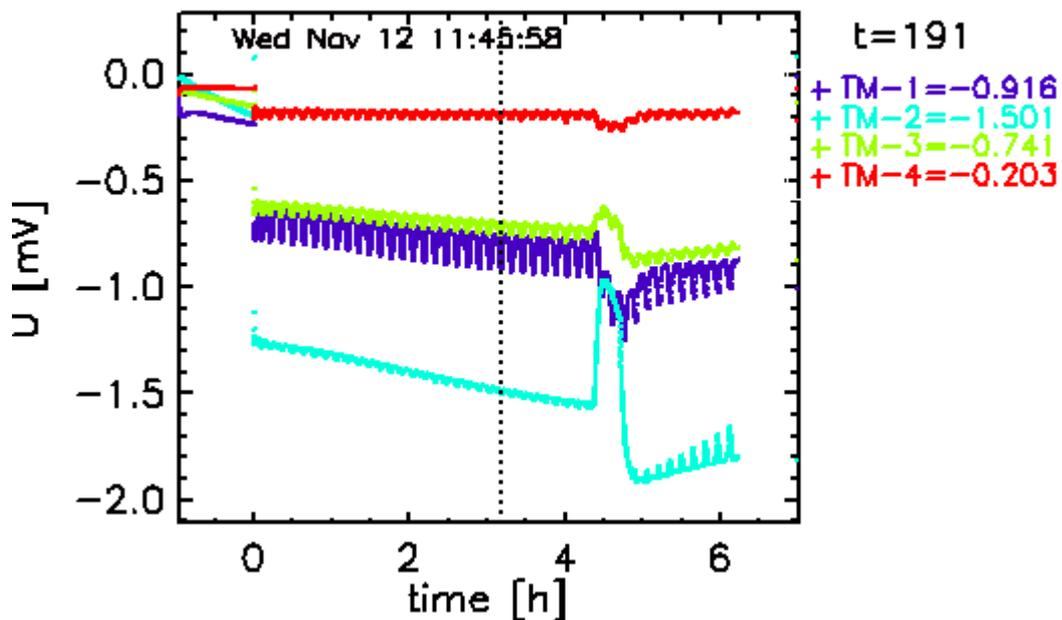
Figure 6-2 TM thermopile signals measured during descent.
