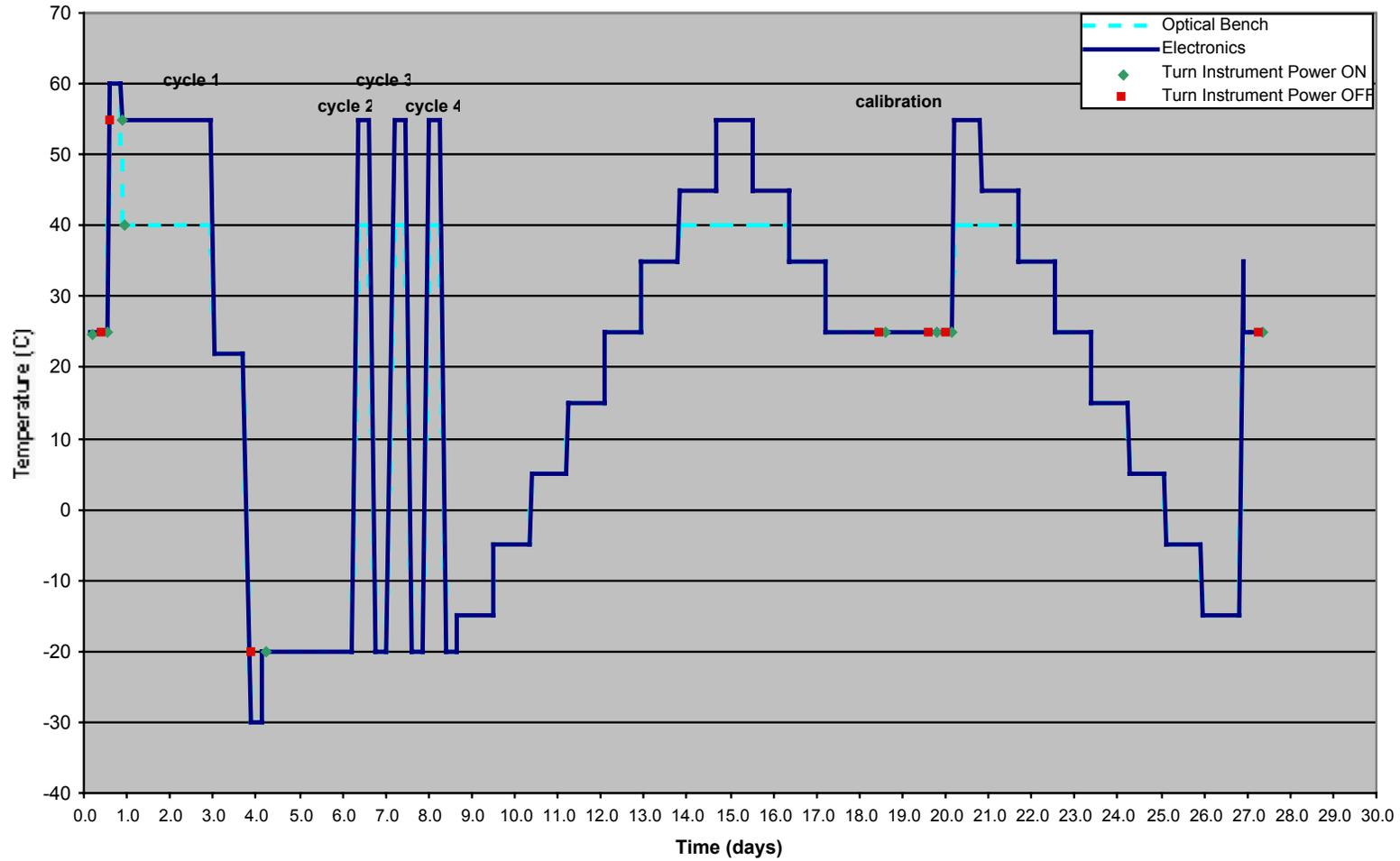
**Figure 1 Thermal/Vacuum Test Profile**
