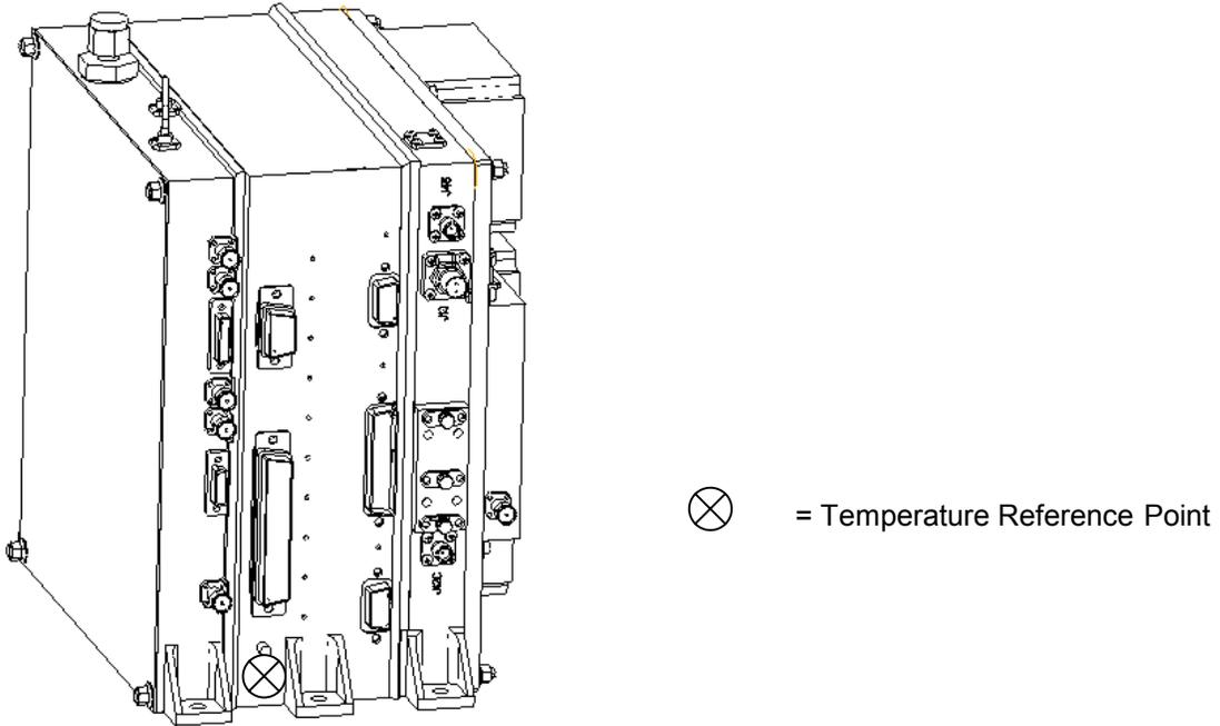
**Figure 3 Sensor Unit Temperature Reference Point**
