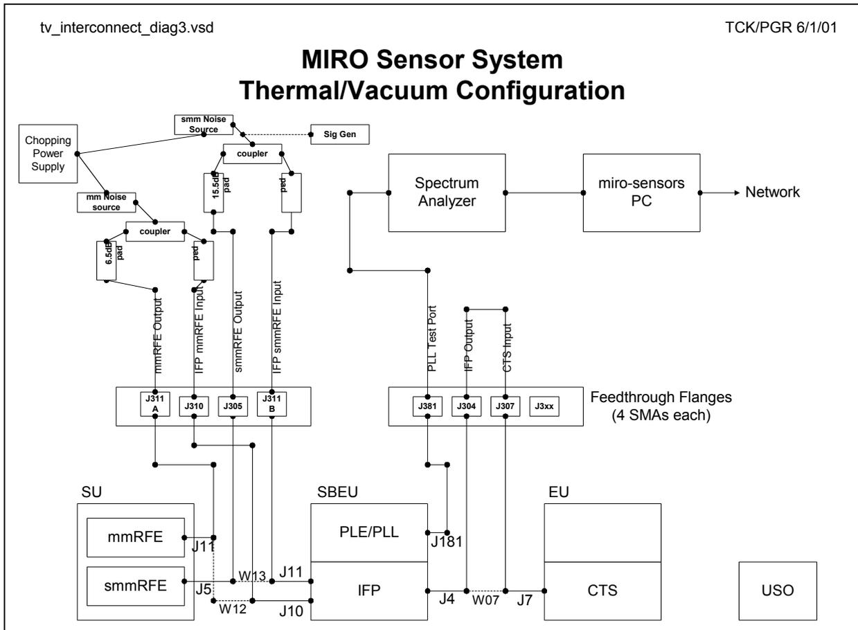
Figure 2: Nominal Recabling of instrument for special tests.
