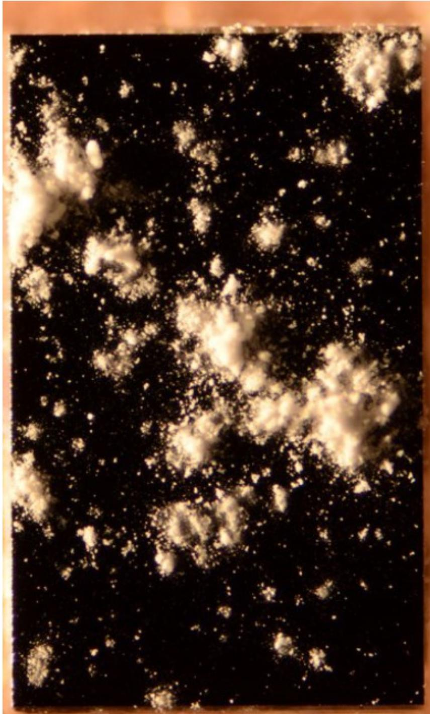
Figure 2.5.4 – M4: 1.5  $\mu\text{m}$  particles fired at 2.7-3.5 m/s.
