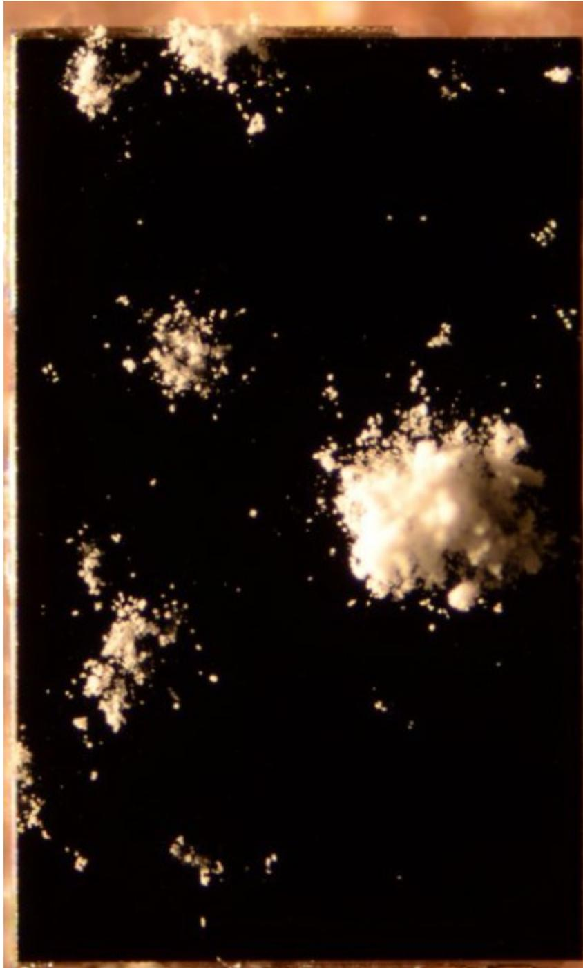
Figure 2.5.5 – M5: 1.5  $\mu\text{m}$  particles fired at 0.2-1.4 m/s.
