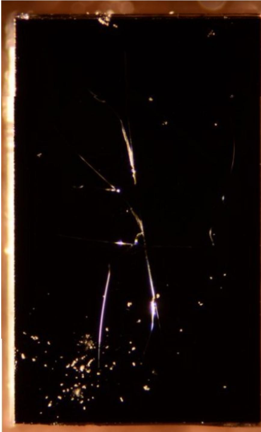
Figure 2.5.7 – M7: 1.0  $\mu\text{m}$  particles fired at 0.8-1.3 m/s.
