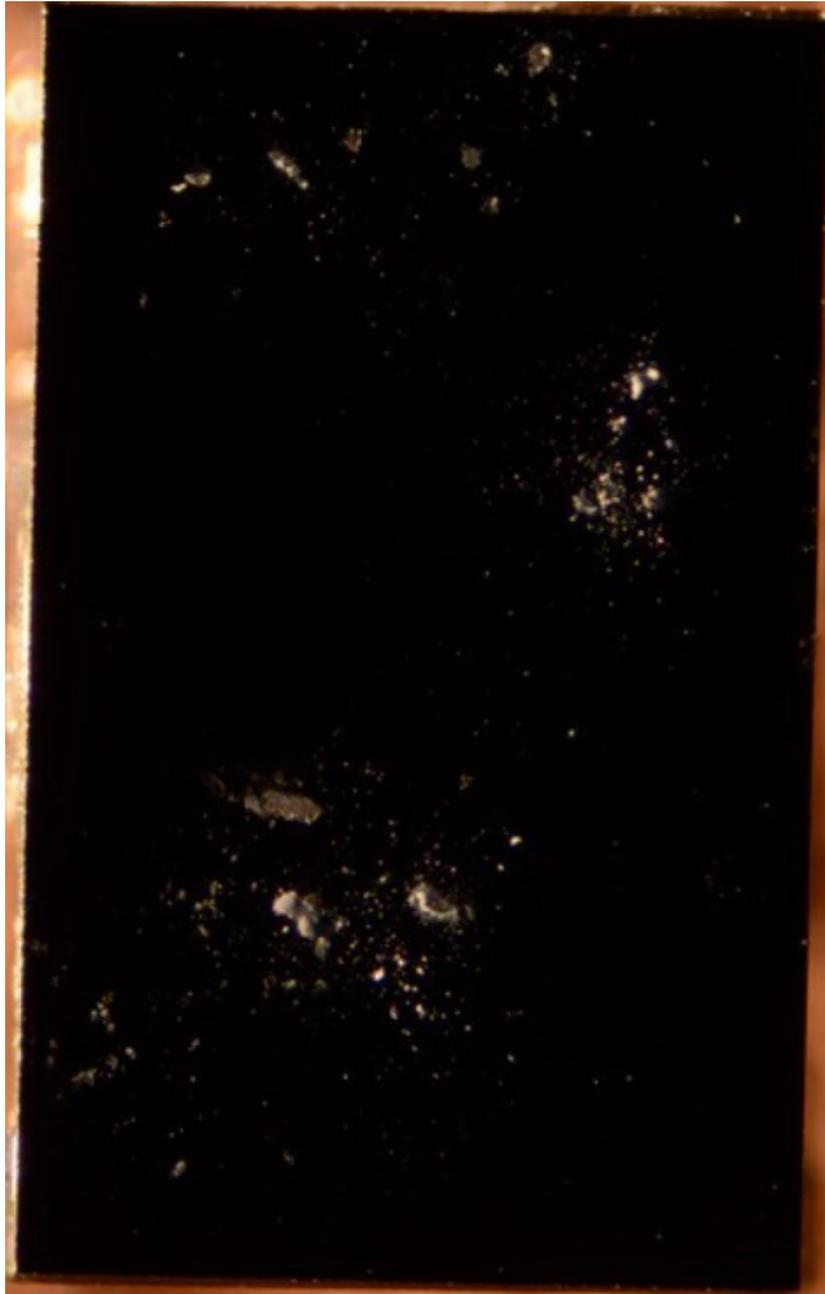
Figure 2.5.2 – M2: 0.3  $\mu\text{m}$  particles fired at 3.6-3.9 m/s.
