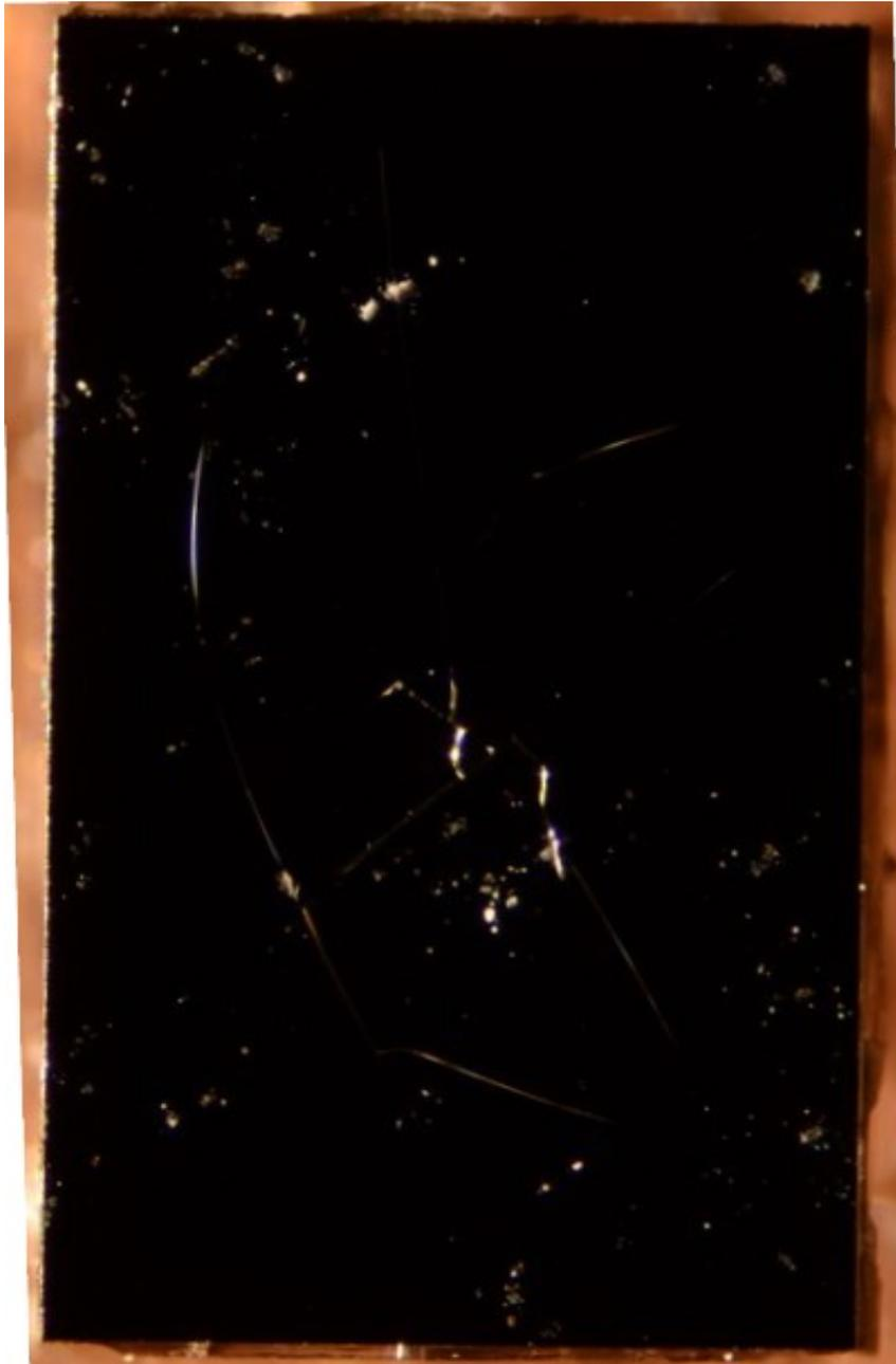
Figure 2.5.3 – M3: 0.3  $\mu\text{m}$  particles fired at 1.1-1.6 m/s.
