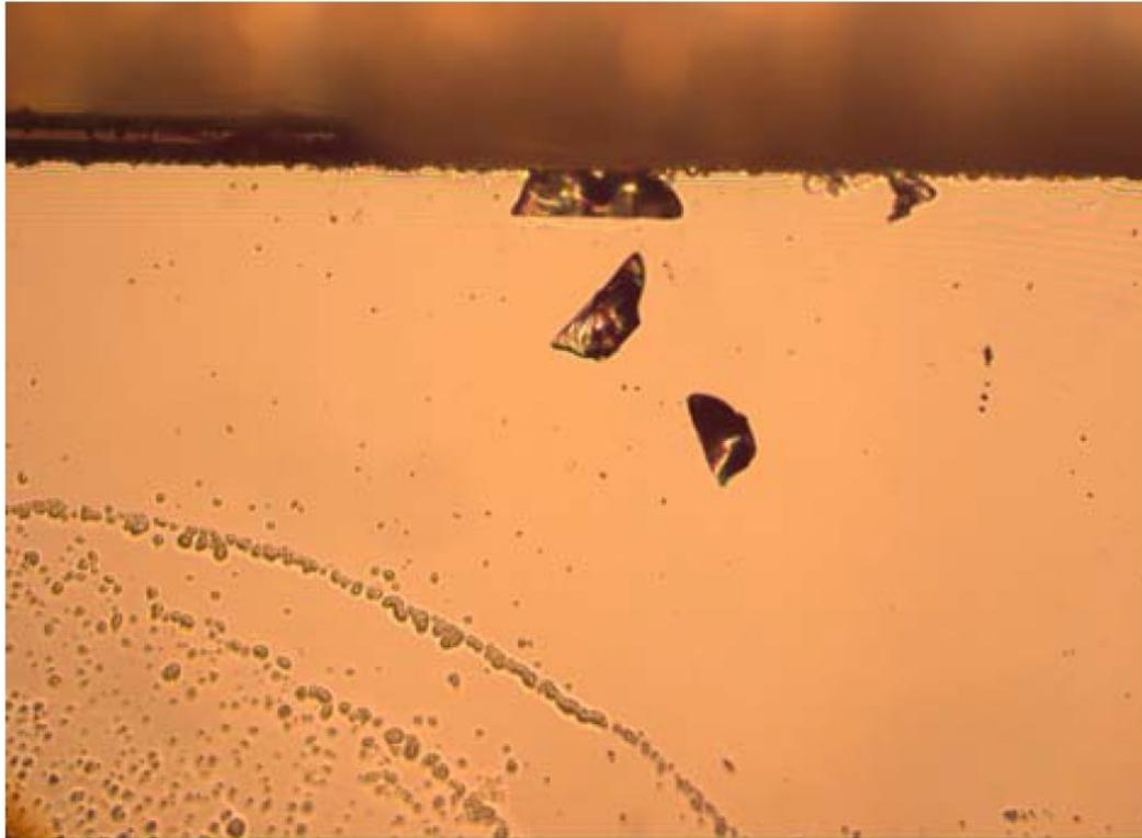
Figure 2.11 - Two particles flaking off the edge of facet 5 ( $710 \mu\text{m} \times 530 \mu\text{m}$ ).
