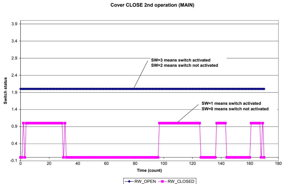
Figure 10 Reed switches Status during Cover Close 2 nd operation @ power-off (MAIN)
