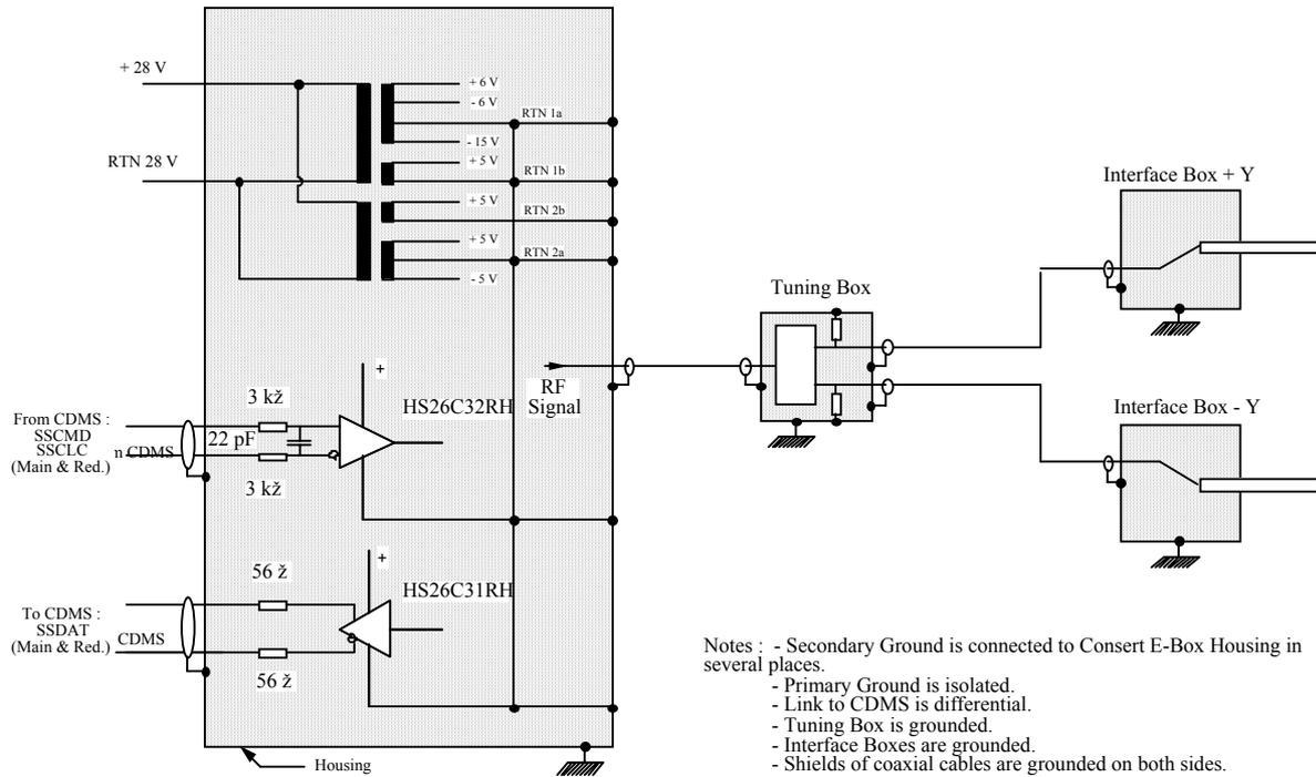
Figure 2.2a. : Lander experiment Grounding Diagram
