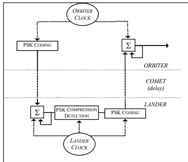
Figure 1.2. : Block diagram of the CONCERT experiment.
