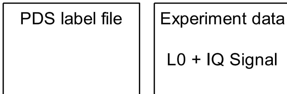
One experiment data file consists in identical records. Each record consists in 3 parts ( 3 x 255 words - Integer 2 bytes): header (named L0), I signal and Q signal. The corresponding data product is organized as three TABLE objects using ROW\_PREFIX\_BYTES and ROW\_SUFFIX\_BYTES for defining the 3 parts.
