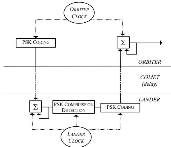
Figure 1 : Block diagram of the CONSERT experiment. The coded signal is emitted from the Orbiter. The Lander makes a coherent addition and a detection of the correlation principal peak. A clean coded signal is finally emitted with the found delay. The Orbiter accumulates the signal and send it to the earth (via the satellite interface).
