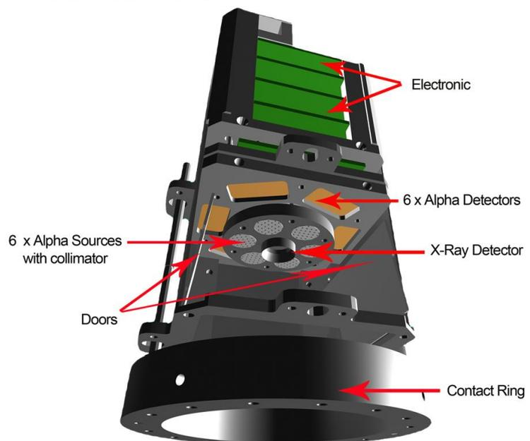
Figure 1 Functional scheme of the APXS sensor head in measurement position. The contact ring is retracted with doors in open position.
