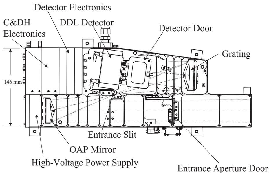
**Figure 2-1: The opto-mechanical layout of *Alice*.**
