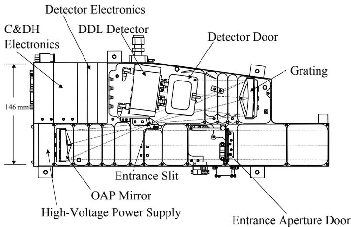
Figure 2-1: The opto-mechanical layout of *Alice*.
