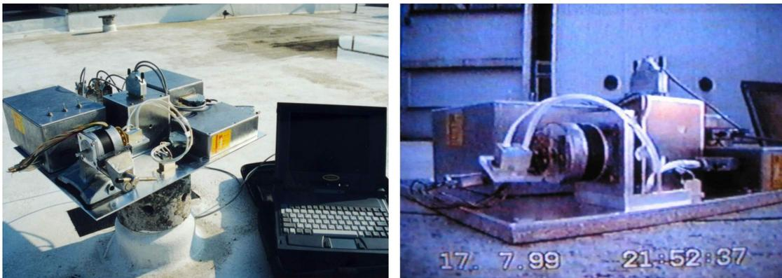
**Figure 4.2: The Portable Dynamic Calibration Platform: early assembly close-up (left), platform on ground at airfield (right)**
