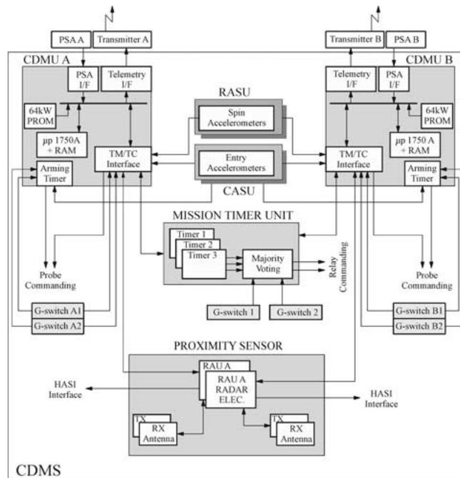
Figure 14. The Probe's Control and Data Management Subsystems (CDMS). CASU: Central Acceleration Sensor Unit; CDMU: Command and Data Management Unit; HASI: Huygens Atmospheric Structure Instrument; I/F: Intermediate Frequency; PSA: Probe Support Avionics; RASU: Radial Acceleration Sensor Unit; TC: Telecommand; TM: Telemetry.
