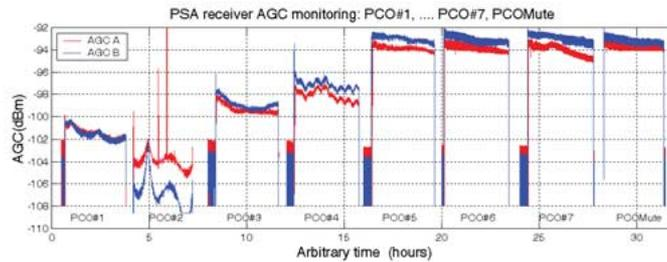
*Figure 20.* This figure illustrates the history of the Huygens receiver AGC signal strength variation during the in-flight checkouts. The strong variation of the AGC observed during the first four checkouts is due to the effect of the solar noise that depends upon the distance to the Sun. The observed modulation during a checkout is due to the spacecraft attitude that modulates the solar noise intensity picked up by Cassini High Gain Antenna.
