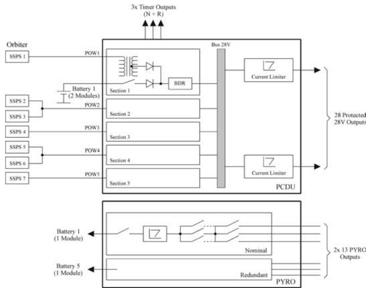
Figure 12. Huygens Probe Electrical Power Subsystem (EPSS). BDR: Battery Discharge Regulator; SSPS: Solid State Power Switch; The power lines (POWs) from the Orbiter to BDR's sections are called: Pow1: SSPS1 to BDR1; POW2: SSPS 2 + SSPS 3 to BDR 2; POW3: SSPS 4 to BDR 3; POW4: SSPS 5 + SSPS 6 to BDR 4; POW5: SSPS 7 to DBR 5.
