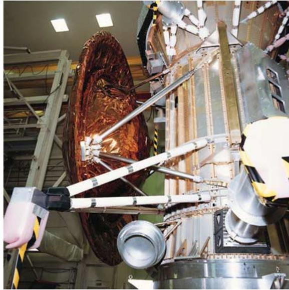
Figure 7. Huygens Probe Accommodation on the Orbiter (A Probe development model and the Orbiter mechanical mock-up model are shown in this figure).
