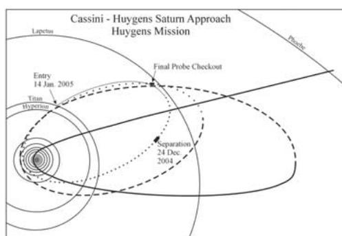
Figure 4. Cassini/Huygens Initial Orbits around Saturn. The Probe mission will be conducted on the third orbit.
