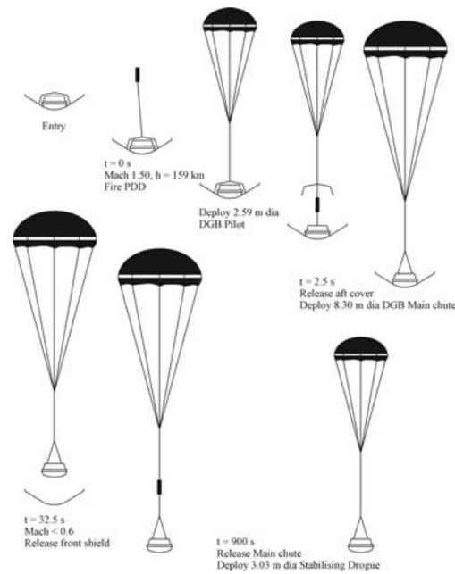
Figure 10. Huygens Parachute Deployment Sequence.
