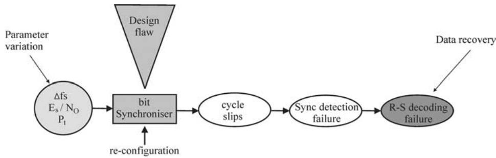
Figure 18. Link anomaly and its consequences which result in data corruption.
