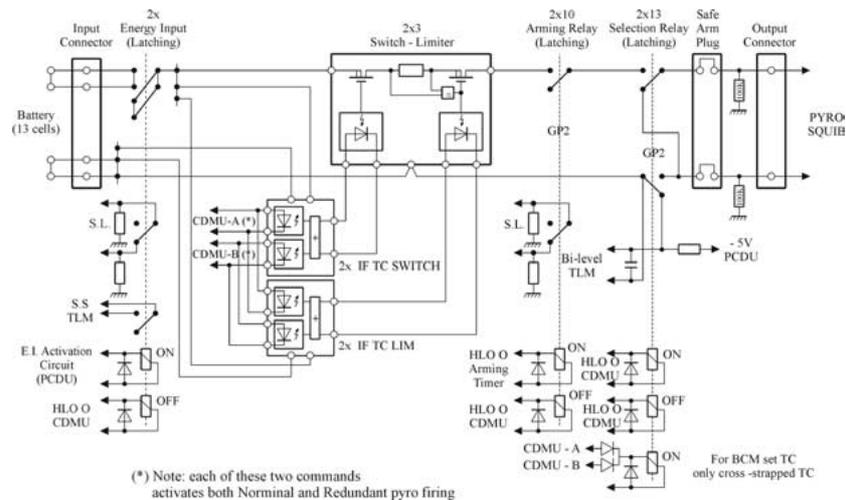
Figure 13. Configuration of the Huygens Probe pyro unit. BCM: Back Cover Mechanism; CDMU: Command and Data Management Unit; HL O/O: High Level On/Off; I/F: Interface; PCDU: Power Conditioning & Distribution Unit; SL: Switch and Limiter; SS: Subsystem; TC: telecommand; TLM: Telemetry.
