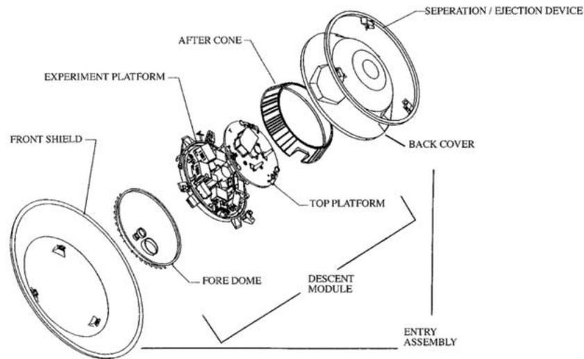
Figure 6. Exploded View of the Huygens Probe. The Huygens Probe comprises the Descent Module (DM) within the Entry Assembly (EA).
