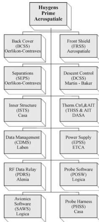
Figure 9. The Huygens Probe Subsystem breakdown.
