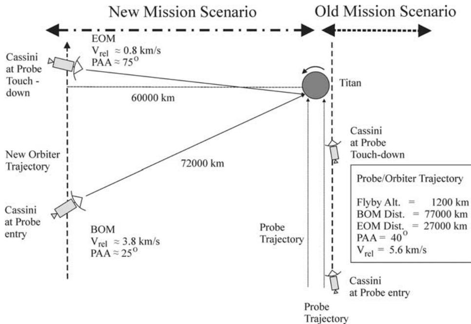
Figure 5. Orbiter trajectory during the Probe mission. For reference, the old baseline trajectory is also indicated.
