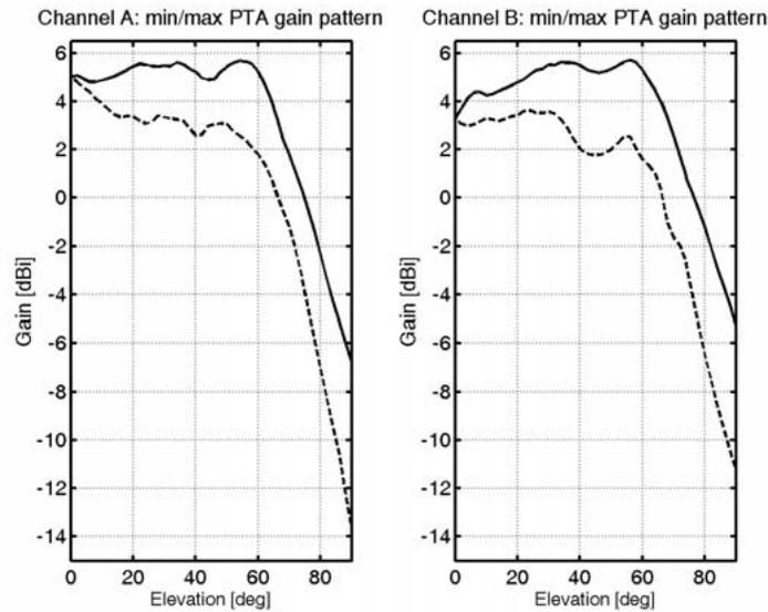
Figure 16. Probe Transmitting antenna pattern envelope as function of the elevation angle.
