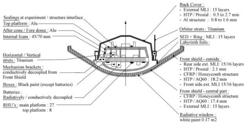
Figure 11. The Probe's thermal control system. RHU: Radioisotope Heater Unit; MLI: Multi Layer Insulation.
