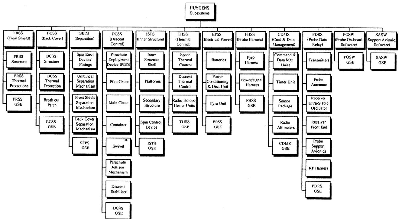
Fig. 7. Huygens Probe subsystem breakdown.
