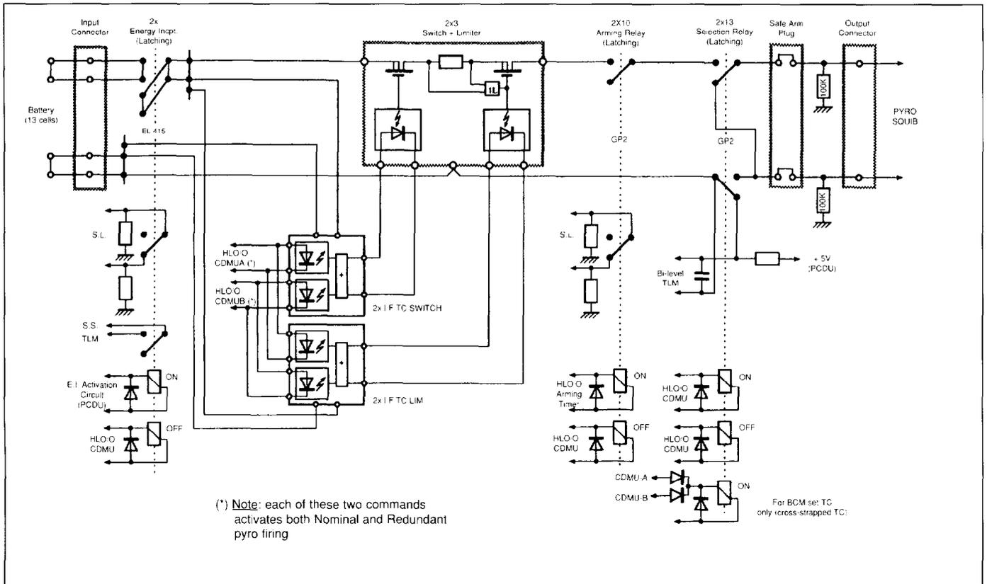
**Fig. 11. Configuration of the Huygens Probe pyro unit.** BCM: Back Cover Mechanism; CDMU: Command and Data Management Unit; HLO/O: High Level On/Off; I/F: intermediate frequency; PCDU: Power Conditioning & Distribution Unit; SL: Switch & Limiter; SS: Subsystem; TC: telecommand; TLM: telemetry.
