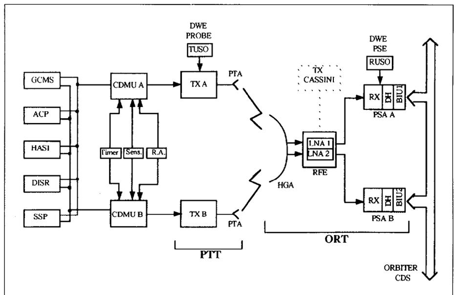
In addition, owing to the HGA's shared use with the Orbiter, a band pass filter (the Tx filter) and a circulator protect the LNA chain B by isolating the Orbiter's S-band transmissions and the Probe's S-band reception, which both use the HGA. These two modes are mutually exclusive.
