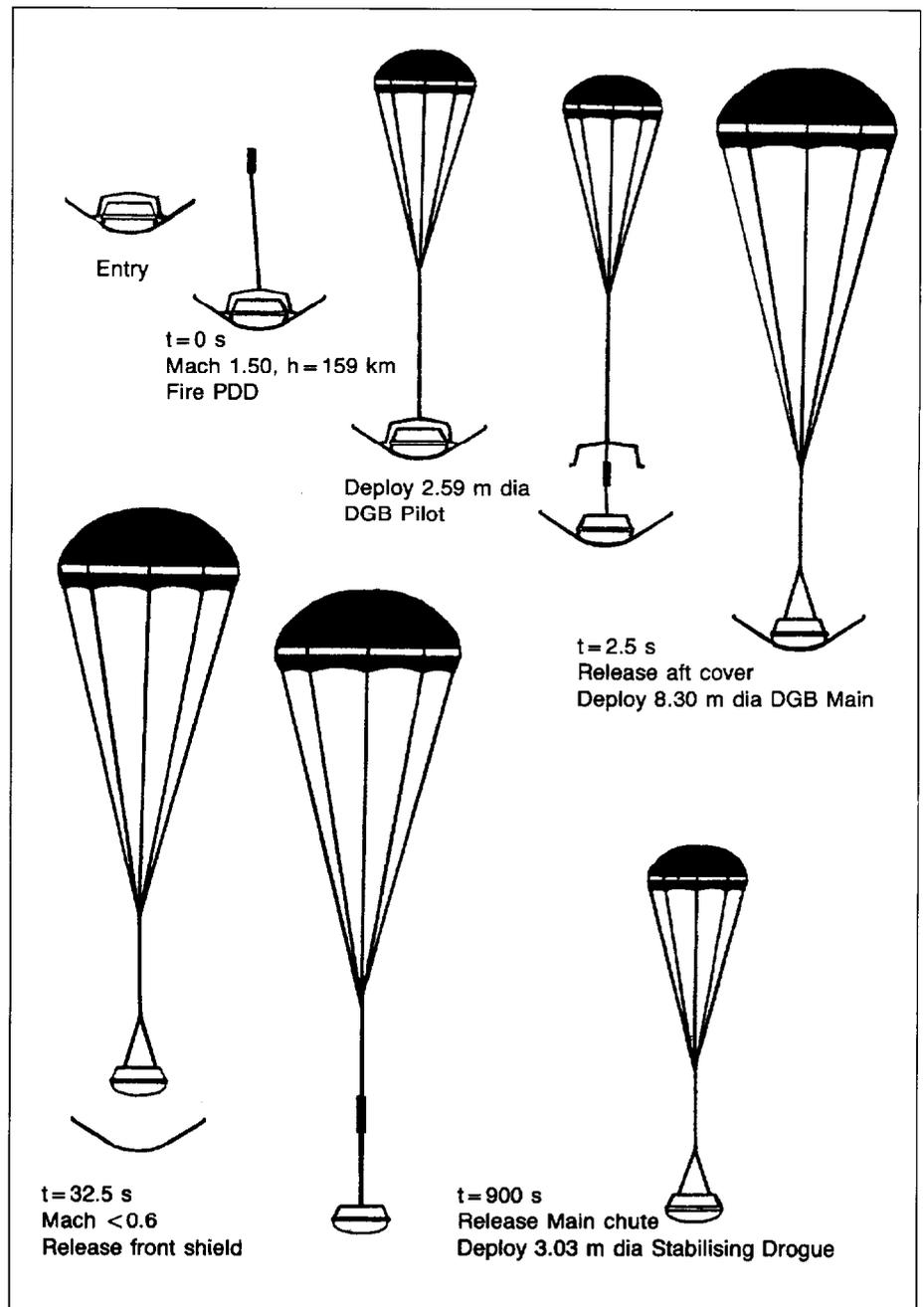
Fig. 8. Huygens parachute deployment sequence.
