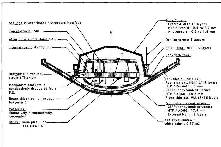
Fig. 9. The Probe's thermal control system.
