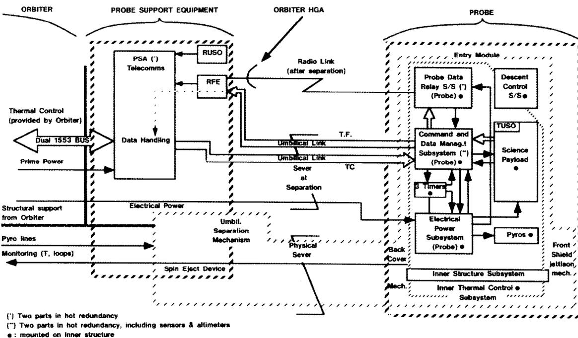
Fig. 5. Huygens Probe System architecture. PSA: Probe System Avionics; S/S: subsystem; TUSO: Transmitter Ultra Stable Oscillator; RUSO: Receiver Ultra Stable Oscillator; HGA: High Gain Antenna; RFE: Receiver Front End; TF: Transfer Frame.
