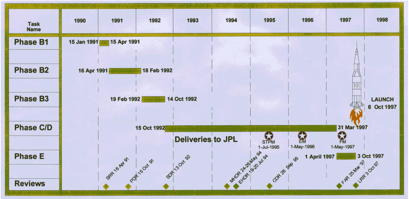
Fig. 3. The Huygens project overall development schedule. SRR: System Requirement Review; PDR: Preliminary Design Review; SDR: System Design Review; MHDR: Mechanical Hardware Design Review; EHDR: Electrical Hardware Design Review; CDR: Critical Design Review; FAR: Flight Acceptance Review; LRR: Launch Readiness Review.
