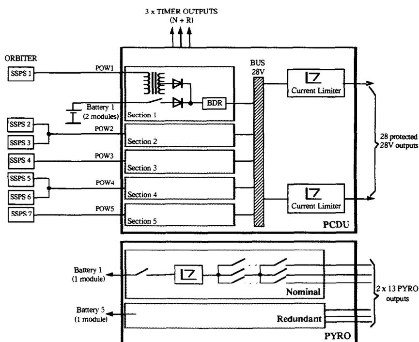
Fig. 10. Huygens Probe Electrical Power Subsystem (EPSS). The power lines (POWs) from the Orbiter to BDR's sections are called: SSPS 1 to BDR 1 = POW1; SSPS 2 + SSPS 3 to BDR 2 = POW2; SSPS 4 to BDR 3 = POW3; SSPS 5 + SSPS 6 to BDR 4 = POW4; SSPS 7 to BDR 5 = POW5. BDR: Battery Discharge Regulator; POW: power line; SSPS: Solid State Power Switch.
