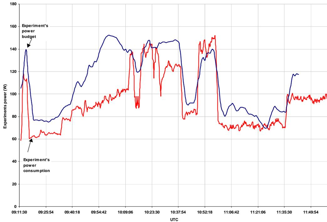
Due to the lost of data from chain A, the power consumption has been estimated from chain B (there are two redundant power buses ored at experiment level). The assumption is that the consumption is balanced on the two buses. This is not true the SSP. The ACP consumption is also different but close to the budget.
