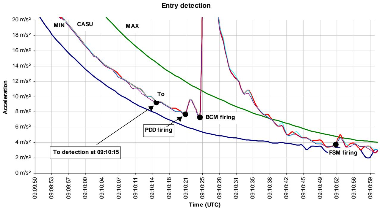
The  $S_0$  event is dated precisely by the chain B “Real Time” and “Mission Time” counters. However it can be observed, thanks to the accelerometer sensors, that the pyro firing orders are around 0.6 s in advance with respect to the theoretical time. This suggests that the  $S_0$  has been detected by chain A first. The 0.6 s interchain delay is below the requirement of 2.2 s max.
