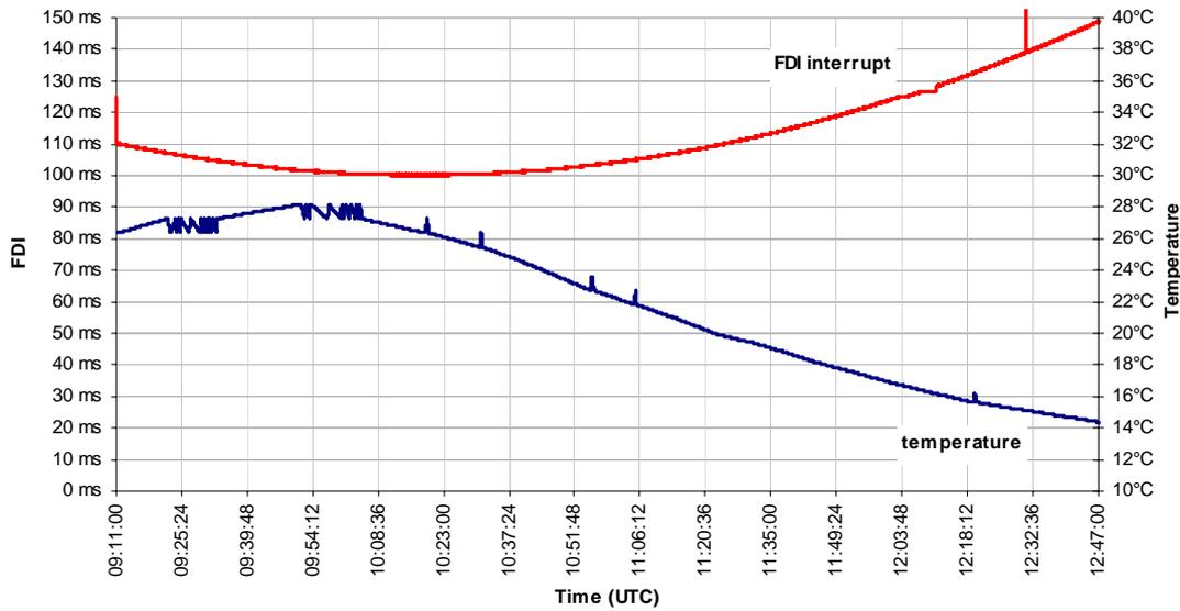
The doppler is the main contributor, but the quartz temperature induces also a frequency drift.
