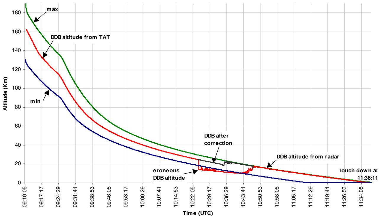
Down to 25 000 Km the DDB altitude was extrapolated from the TAT. Then the two radars were selected as they were locked but providing incorrect altitude. Below 22 000 Km the RAU B provided correct data but was not selected as RAU A was still incorrect. Below 18 000 Km the two radars worked well and the DDB altitude was accurate.
