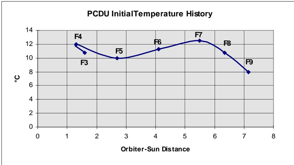
Fig 4.12 : initial PCDU temperature evolution
