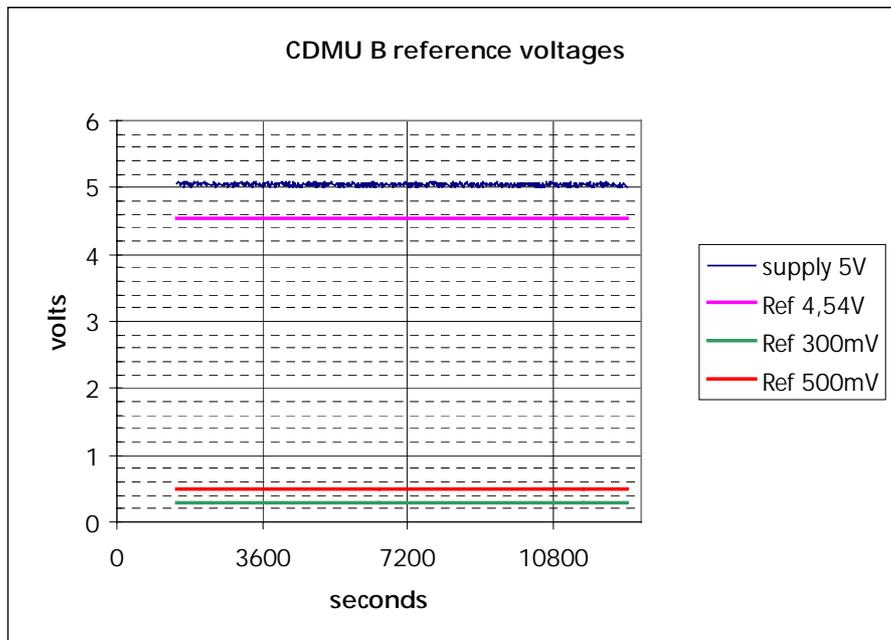
Fig 4.10 : CDMU B Voltages (5V is not stabilized)
