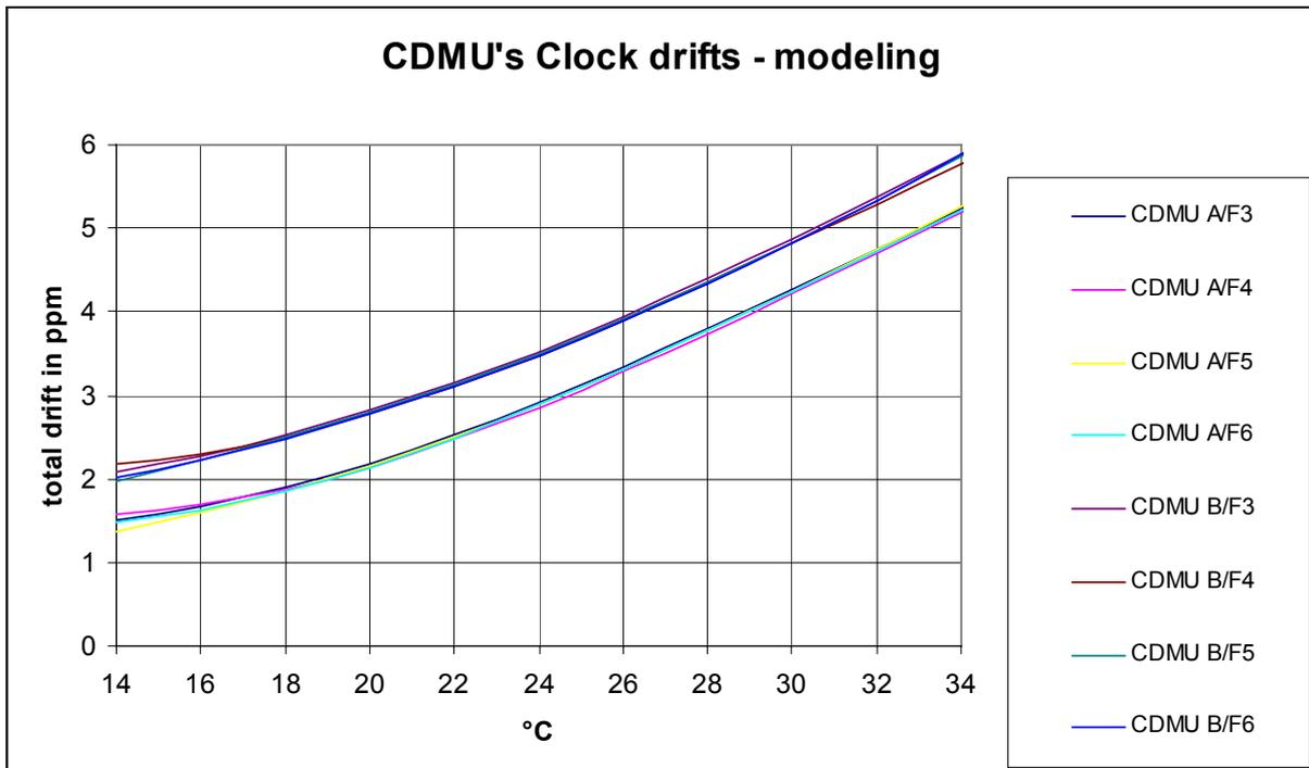
**Fig 4.9 : CDMU A & B TM clock drift over temperature**
