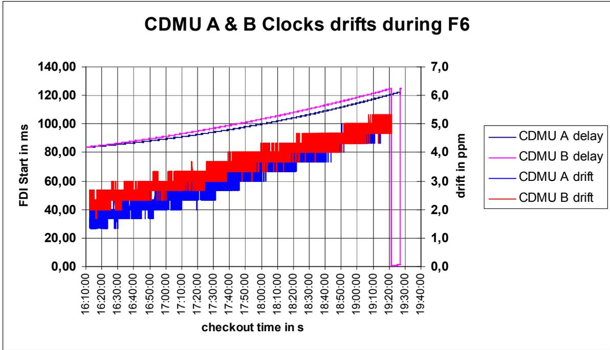
**Fig 4.8 : CDMU A & B TM clock drift over F6**
