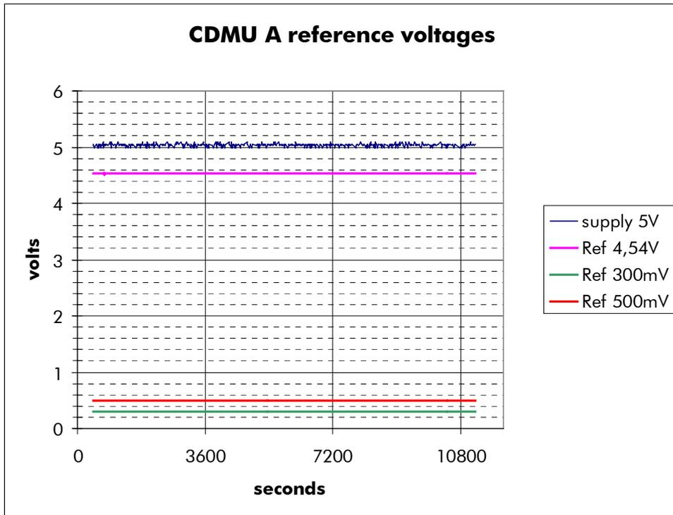
**Fig 4.6 : CDMU A Voltages (5V is not stabilized)**
