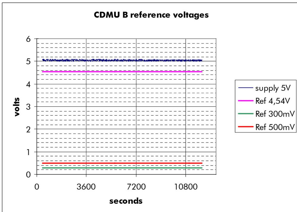
**Fig 4.7 : CDMU B Voltages (5V is not stabilized)**
