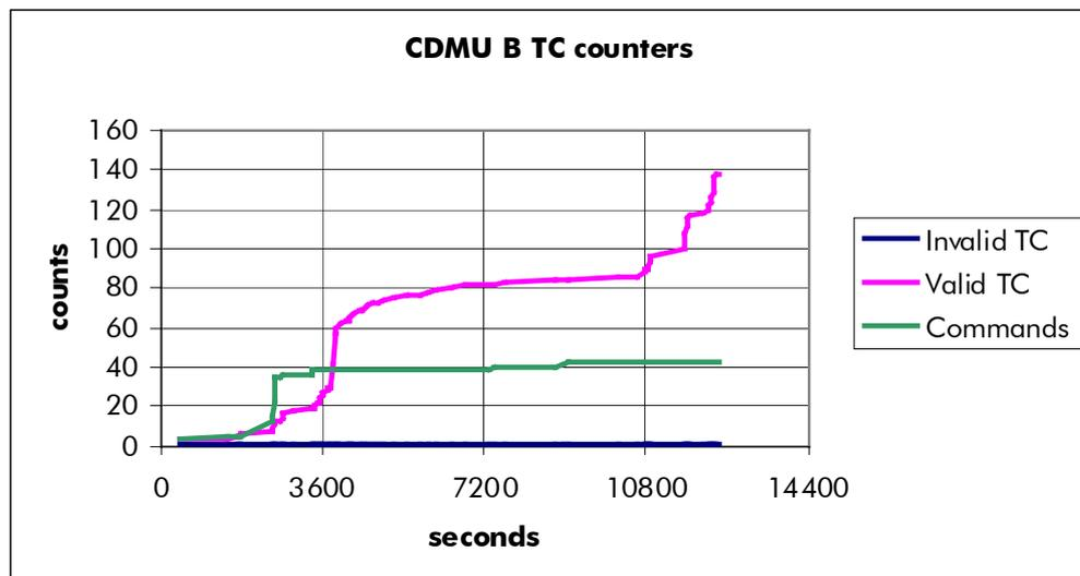
**Fig 4.2 : Telecommand counters telemetry**
