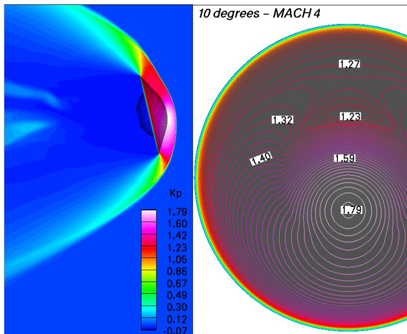
SURFACE PRESSURE COEFFICIENTS DISTRIBUTION AT MACH 4,  $\alpha = 10^\circ$
