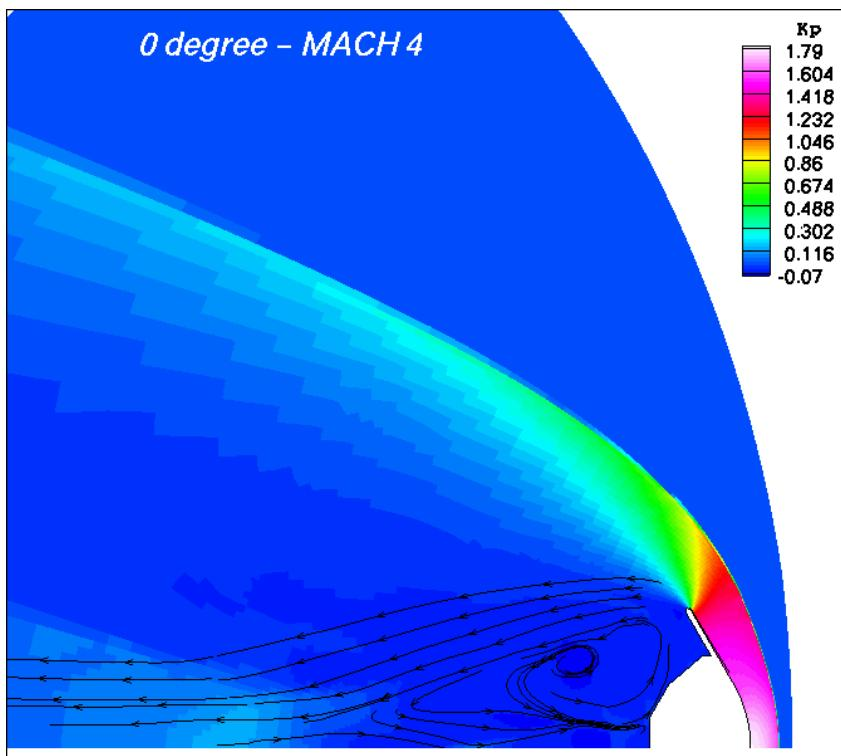
WAKE STRUCTURE AT MACH 4,  $\alpha = 0^\circ$
