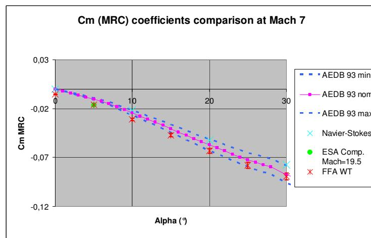
**FIGURE 9 - TEST AND CFD COMPUTATIONS VS. PREVIOUS AEDB FOR PITCHING MOMENT COEFFICIENT AT MRC AND AT MACH 7**
