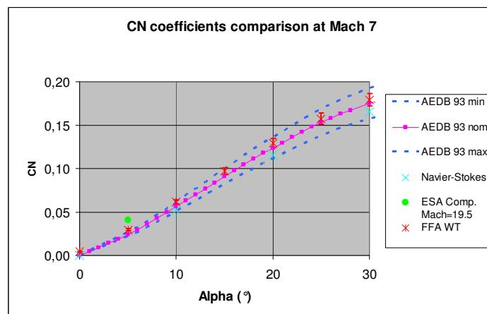
**FIGURE 8 - TEST AND CFD COMPUTATIONS VS. PREVIOUS AEDB FOR NORMAL FORCE COEFFICIENT AT MACH 7**
