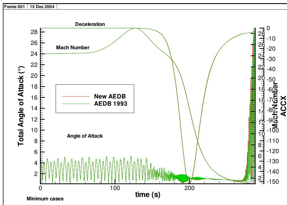
**FIGURE 18 -  $\gamma E = -68^\circ$  YELLE MINIMUM DENSITY: FLIGHT MECHANICS PARAMETERS**
