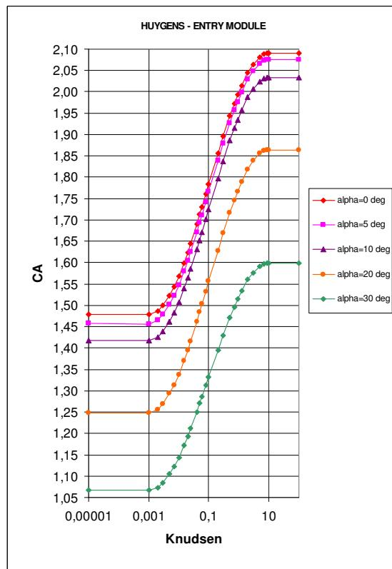
**FIGURE 10 -  $C_A$  COEFFICIENTS VERSUS KNUDSEN NUMBER AND  $\alpha$**
