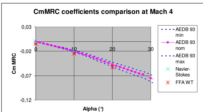
**FIGURE 6 - TEST AND CFD COMPUTATIONS VS PREVIOUS AEDB FOR PITCHING MOMENT COEFFICIENT AT MRC AND AT MACH 4**
