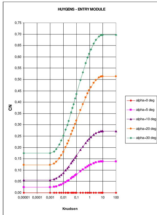
FIGURE 11 -  $C_N$  COEFFICIENTS VERSUS KNUDSEN NUMBER AND  $\alpha$
