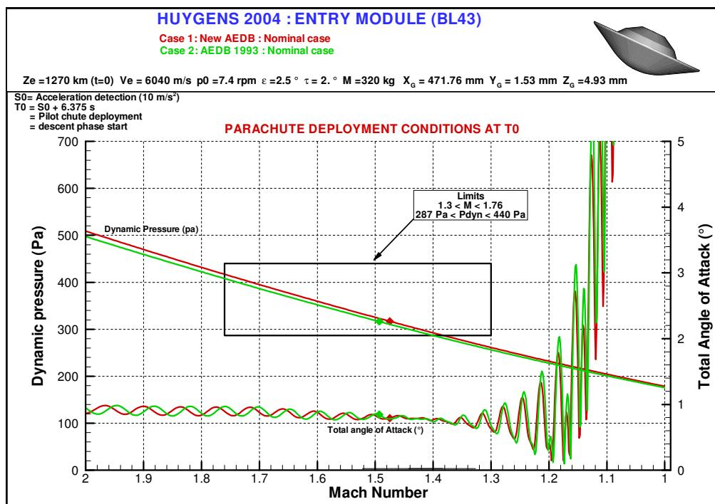
**FIGURE 15 -  $\gamma_E = -65^\circ$  YELLE NOMINAL DENSITY: PDD CONDITIONS**
