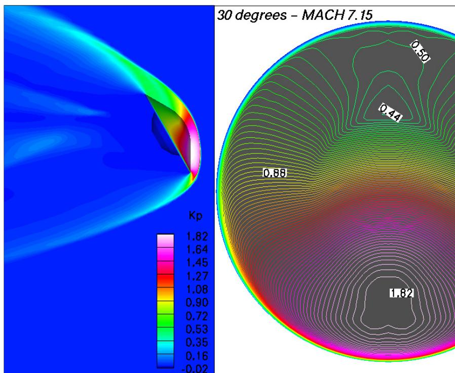
SURFACE PRESSURE COEFFICIENT DISTRIBUTION AT MACH 7.15,  $\alpha = 30^\circ$
