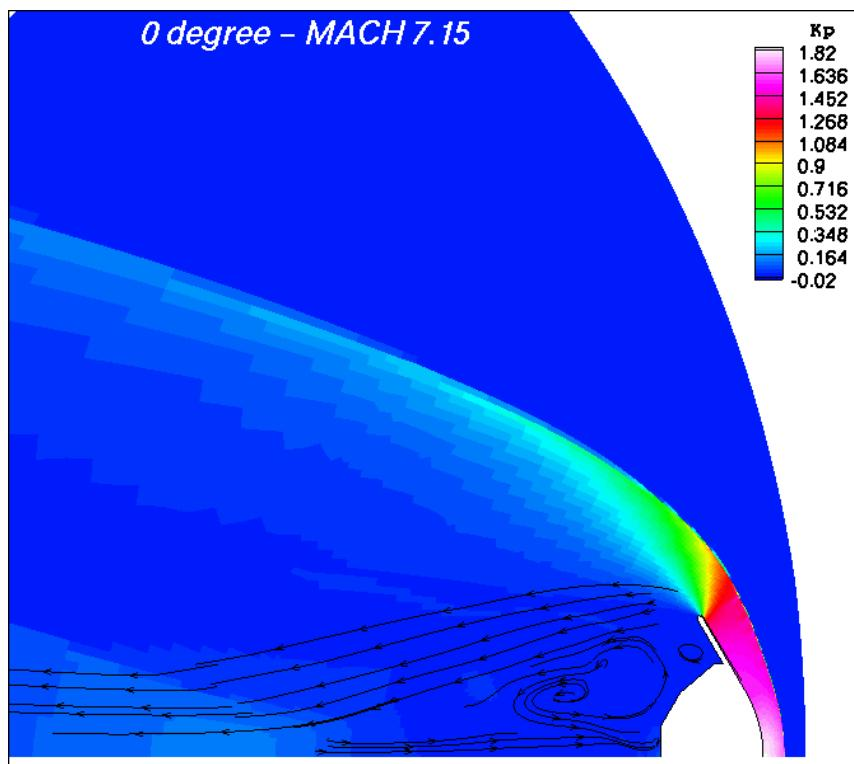
WAKE STRUCTURE AT MACH 7.15,  $\alpha = 0^\circ$
