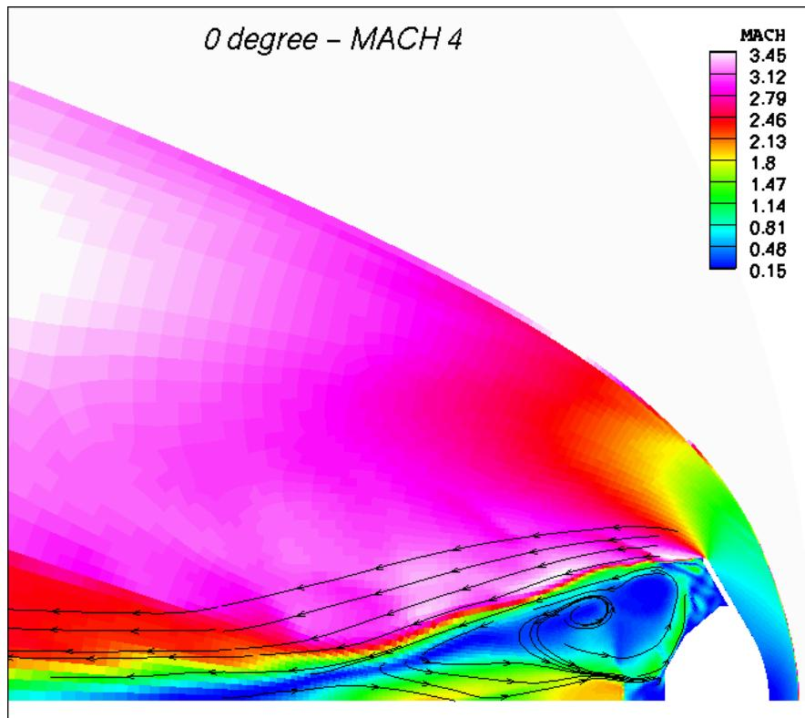
WAKE STRUCTURES AT MACH 4,  $\alpha = 0^\circ$
