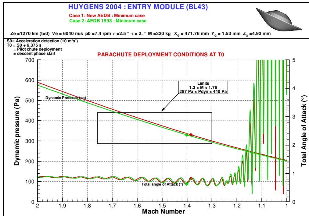
**FIGURE 17 -  $\gamma E = -68^\circ$  YELLE MINIMUM DENSITY: PDD CONDITIONS**
