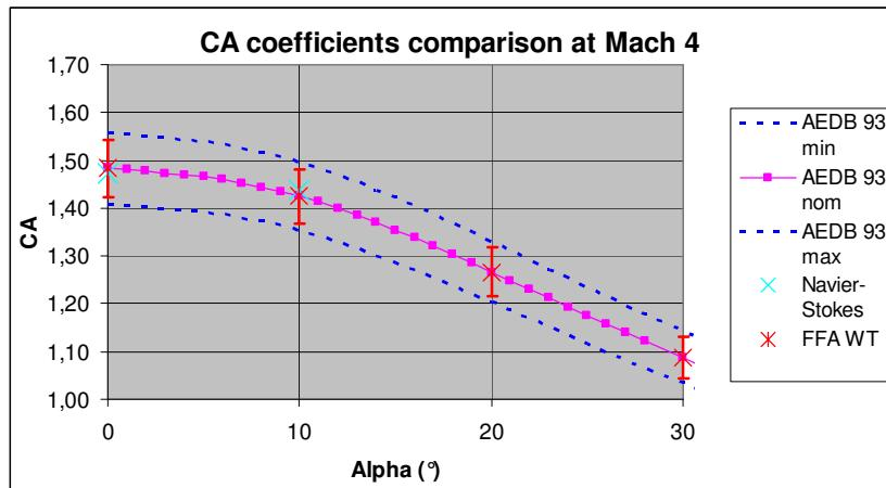
**FIGURE 4 - TEST AND CFD COMPUTATIONS VS. PREVIOUS AEDB FOR AXIAL FORCE COEFFICIENT AT MACH 4**
