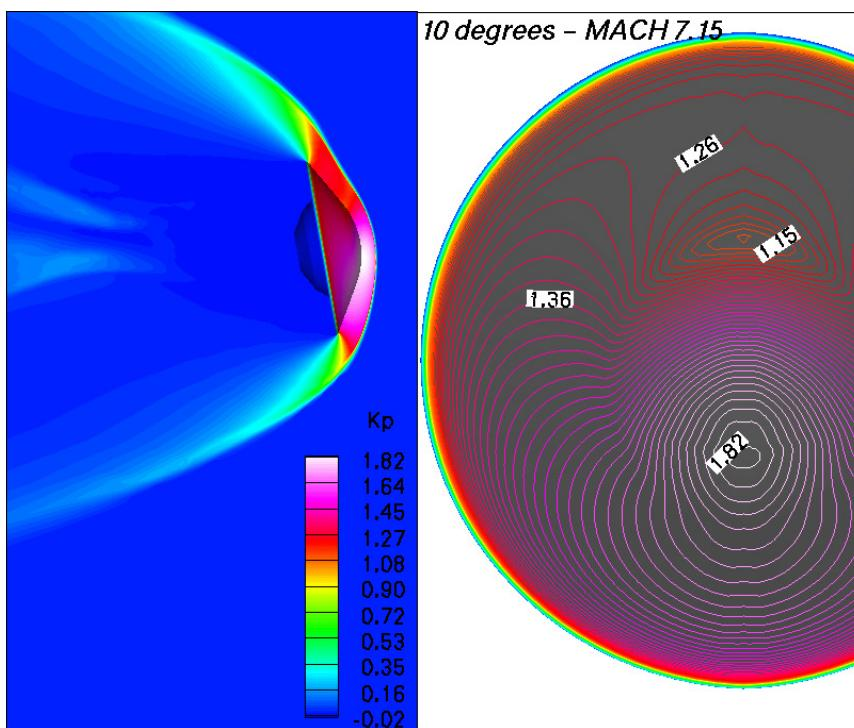
SURFACE PRESSURE COEFFICIENT DISTRIBUTION AT MACH 7.15,  $\alpha = 10^\circ$
