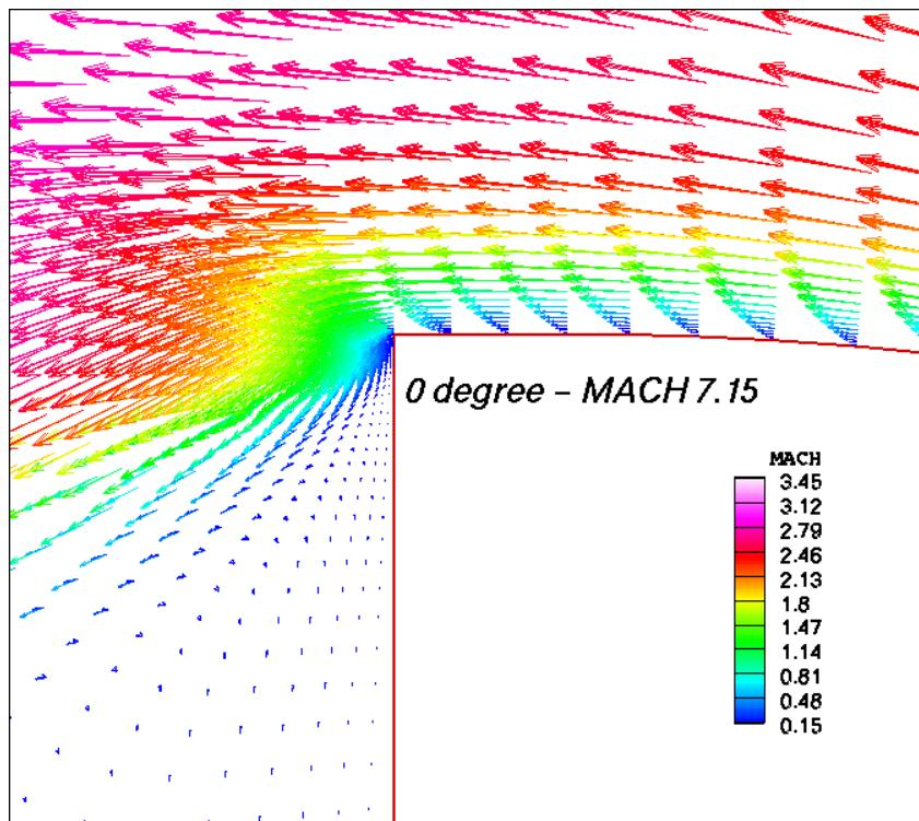
FLOW DETAILS AT SHOULDER SEPARATION AT MACH 7.15,  $\alpha = 0^\circ$
