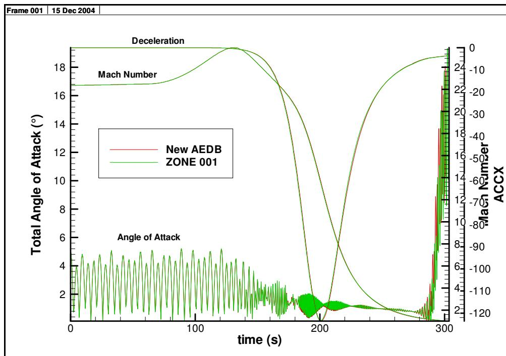
**FIGURE 16 -  $\gamma_E = -65^\circ$  YELLE NOMINAL DENSITY: FLIGHT MECHANICS PARAMETERS**
