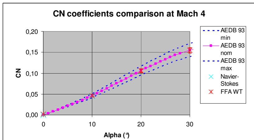
**FIGURE 5 - TEST AND CFD COMPUTATIONS VS. PREVIOUS AEDB FOR NORMAL FORCE COEFFICIENT AT MACH 4**
