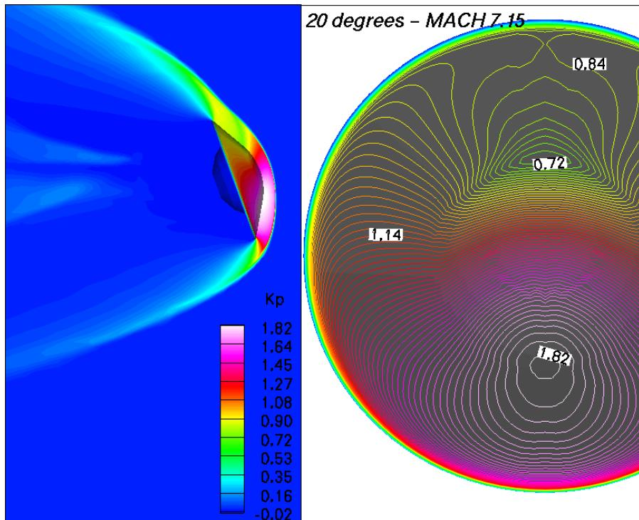
SURFACE PRESSURE COEFFICIENT DISTRIBUTION AT MACH 7.15,  $\alpha = 20^\circ$
