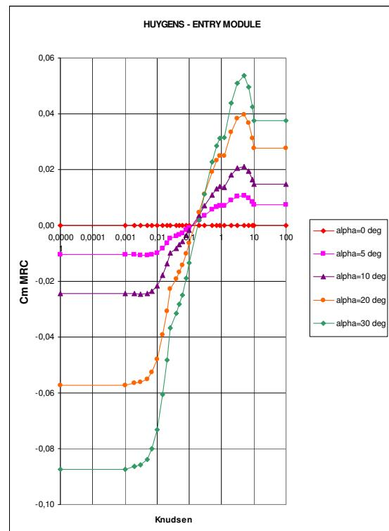
FIGURE 12 -  $C_{mMRC}$  COEFFICIENTS VERSUS KNUDSEN NUMBER AND  $\alpha$
