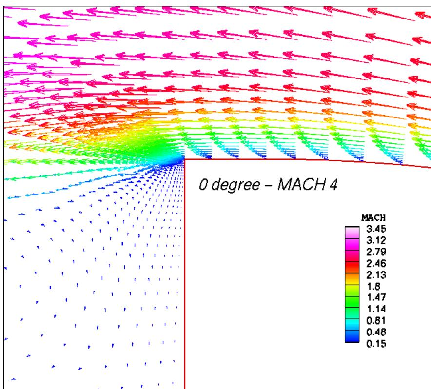
FLOW DETAILS AT SHOULDER SEPARATION AT MACH 4,  $\alpha = 0^\circ$
