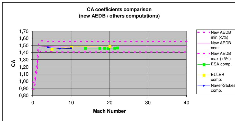
**FIGURE 14 - NEW DATABASE/OTHER COMPUTATION RESULTS COMPARISON ( $\alpha = 0^\circ$ )**
