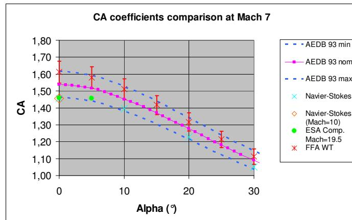
**FIGURE 7 - TEST AND CFD COMPUTATIONS VS. PREVIOUS AEDB FOR AXIAL FORCE COEFFICIENT AT MACH 7**
