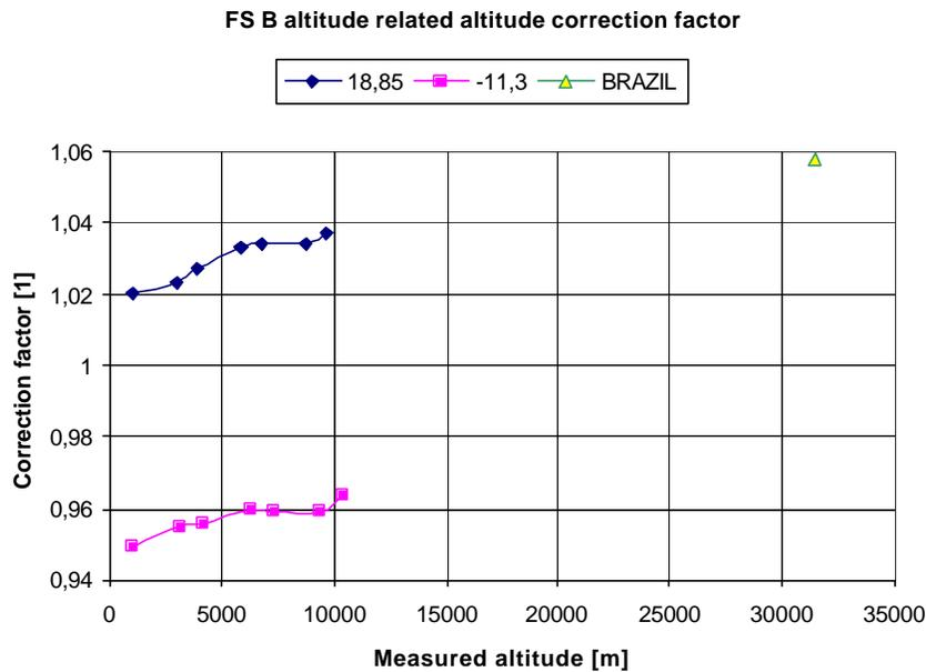
**Figure 6: FS B relative altitude error vs. altitude (parameter: temperature)**
