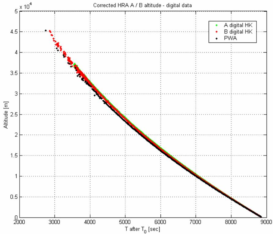
**Figure 2: Digital interface altitude data after digital error correction**
