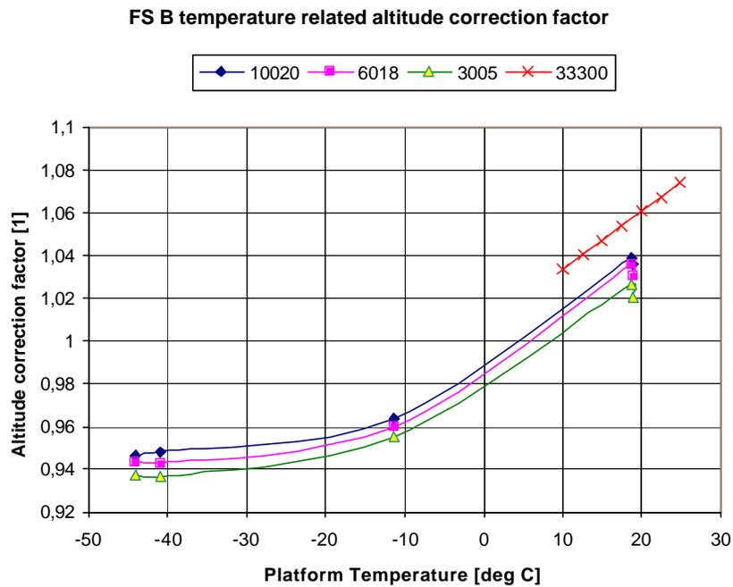
Figure 5: FS B temperature related altitude correction factor (parameter: altitude)
