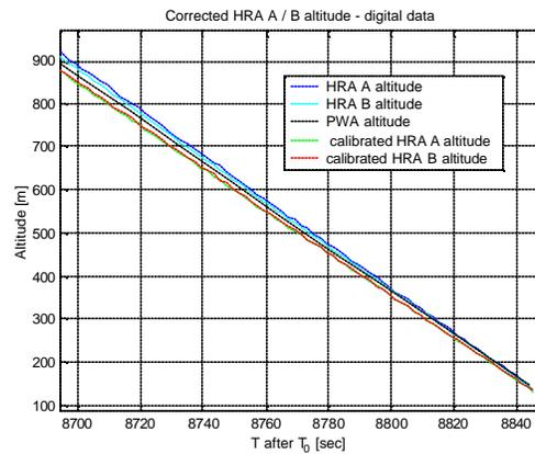
Figure 13: Uncorrected and corrected digital HRA data – detail 3
