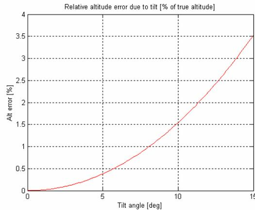
**Figure 9: Relative altitude measurement error vs. probe tilt angle**
