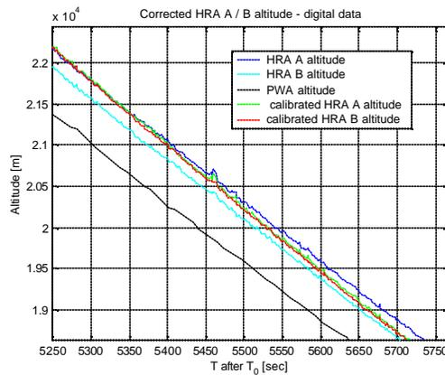
Figure 12: Uncorrected and corrected digital HRA data – detail 2
