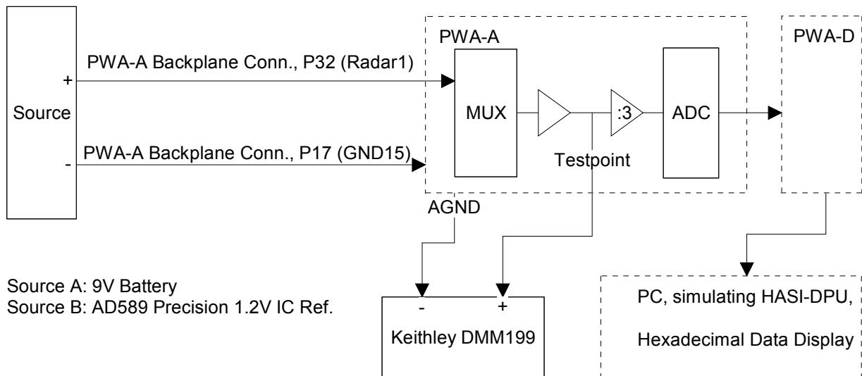
Measured attenuator gain:
