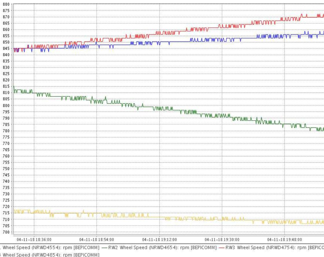
Figure 1 : Reaction wheel frequencies vs. time during the time of the rate test.
