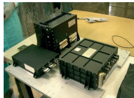
Fig. 12. The VIRTIS electronics boxes shortly before integration at IAS Orsay, Paris, during the calibration campaign at the beginning of 2004. The main electronics are at top, PEM-H is at left and PEM-M is at right.
