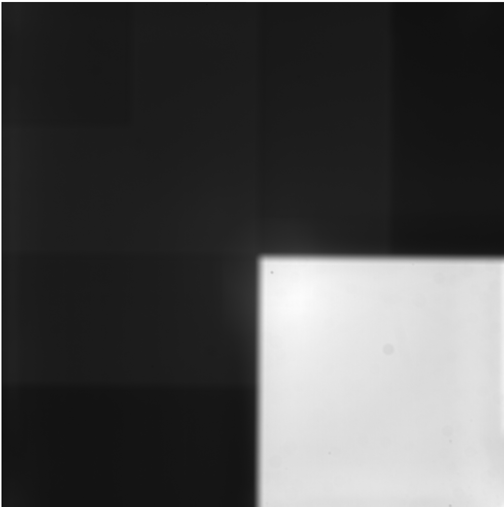
Figure 19: The flat field computed from laboratory images. The gray scale is adapted to the NONE filter area.
