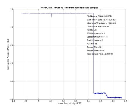
Record Length: 8260 Number of Records: 2880 Sample Rate: 2000 Sample Bits: Start Time: 2016-12-31T02:52:01 Stop Time: 2016-12-31T03:40:00 DSS Receive Antenna: 15 RSR ID: 06 RSR Subchannel: 1 Spacecraft ID: 41 Downlink Band: Х Tracking Mode: Orbit Number: 16466
