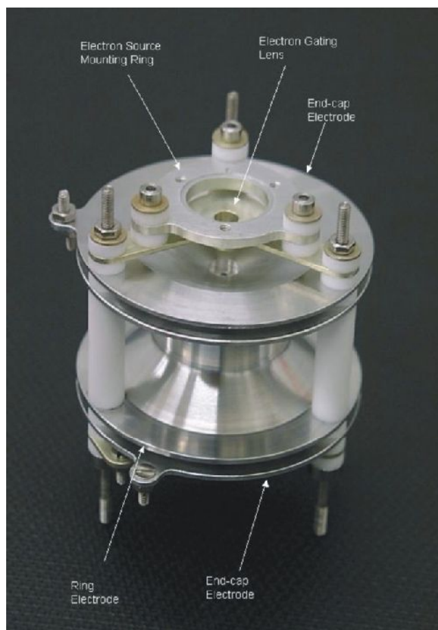
Figure 2. Photograph of the assembled electrodes of the flight model (FM) of the Ptolemy ion trap. The electrodes are fabricated from aluminium; the electron source and detector are each mounted on supports, one of which is shown above the upper end-cap. The total mass of the electrode assembly together with the ion source and detector is 75 g. (Copyright CCLRC Rutherford Appleton Laboratory, reproduced with permission).
