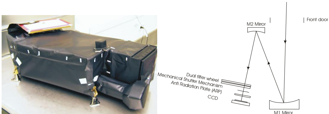
Figure 2 (left) The OSIRIS WAC flight unit in the lab. (right) The WAC Optical path
