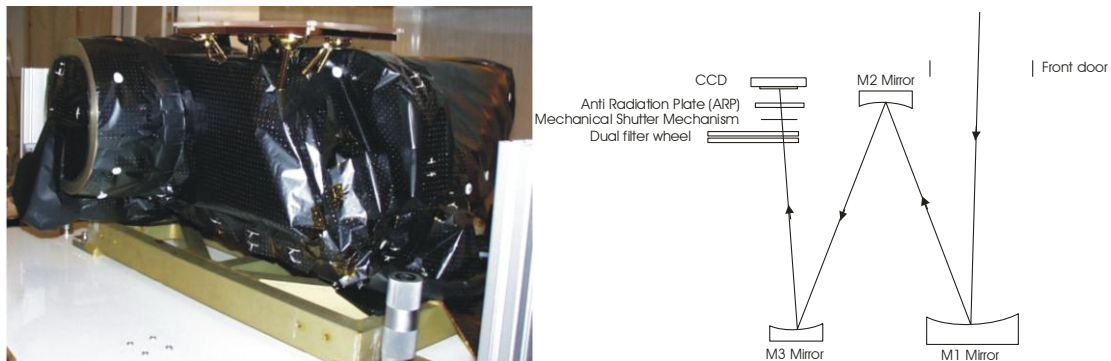
Figure 1 (right) The OSIRIS NAC flight unit in the lab. (left) The NAC Optical path
