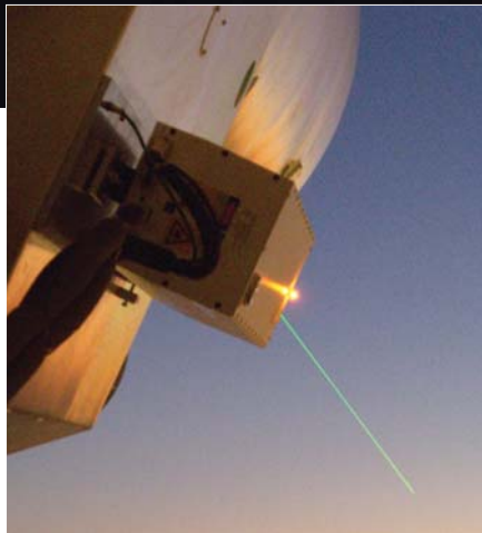
Green laser at dawn for a TerraSAR-X link test
