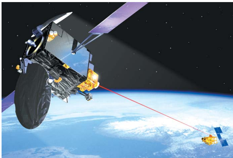
Spot-4 (right) beams its data to the SILEX terminal aboard Artemis along the laser link
