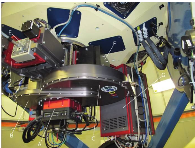
FIG. 5.—Sinistro instrument package mounted on the tailpiece of a 1 m telescope. (A) SBIG STX-16803 4\text{ K} \times 4\text{ K} CCD camera. (B) Rotating-disk shutter assembly. (C) 3-layer filter wheel assembly. (D) Side port with independent focus stage for LIHSP camera or autoguider. (E) Andor Luca S LIHSP camera; may also be used as autoguider. (F) Side port (one of 4) with blank-off panel. (G) Electronics crate for tailpiece power distribution, signal conditioning, and related functions.
