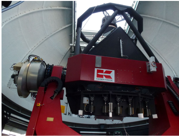
Fig. 1 WWFI ( left ) mounted at one Nasmyth port of the Fraunhofer Telescope
