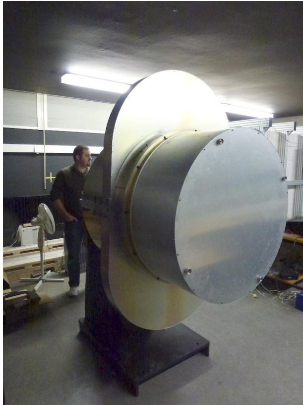
Figure 4. WWFI EMI proof cover: WWFI mounted on test flange in USM lab. All chromated covers attached.
