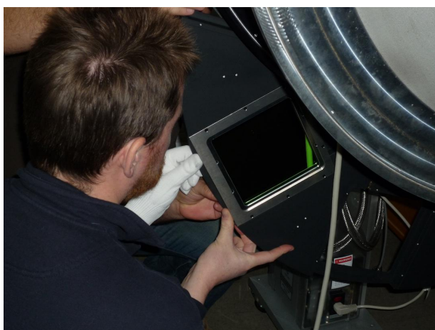
Figure 3. Pictures of WWFI integration. Top left: Main WWFI truss with filter wheels and tip-/tilt stage for the SI900. Top right: Flexure test of the truss shows that flexure is well within specs. Bottom left: Test insertion of filter within its cartridge. Bottom right: SI900 within our optical test bench. Proof of concept for the heat exchangers of the controller and detector compartment (CDC).
