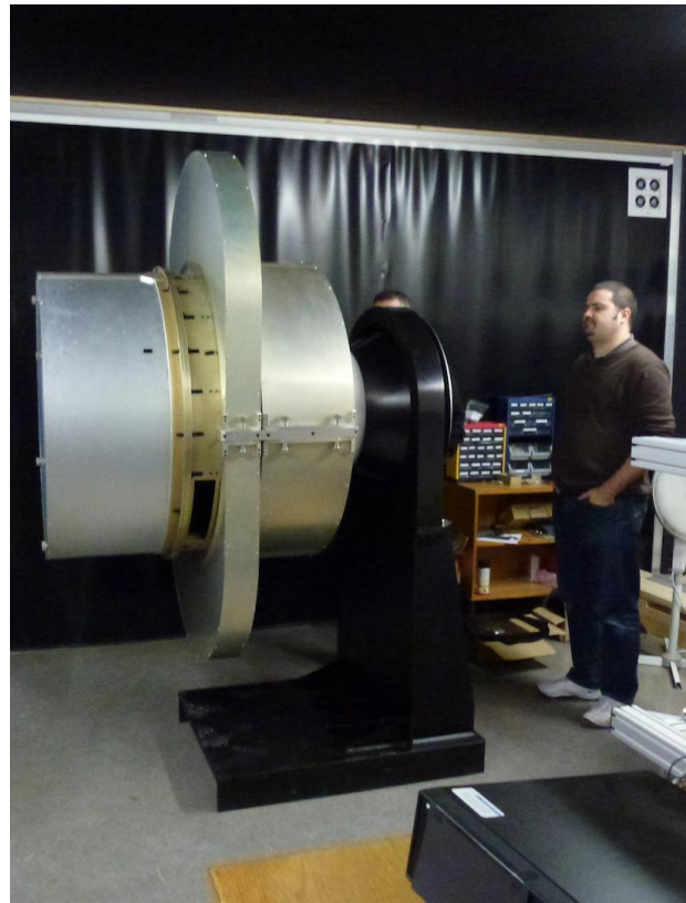
Figure 4. WWFI EMI proof cover: WWFI mounted on test flange in USM lab. All chromated covers attached.
