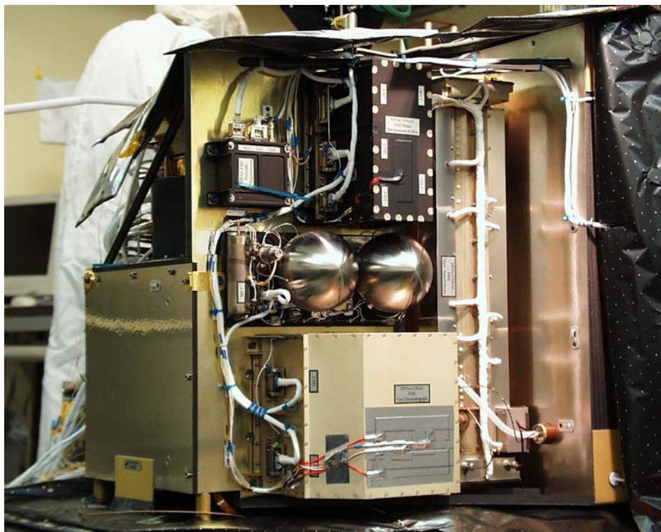
Figure 1. The complete COSAC instrument (apart from the tapping stations) as integrated on Philae. It is approximately 400 mm wide and 500 mm tall.
