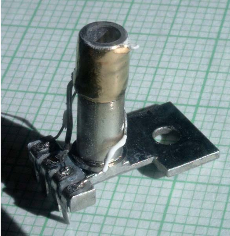
Figure 10. A high temperature oven (HTO) of Philae. Such ovens may be connected to Ptolemy or COSAC.
