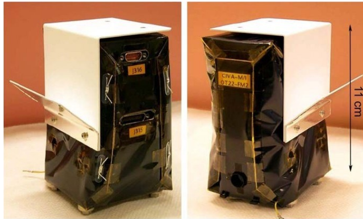
Figure 5 CIVA-M/I FM prior to implementation on Philae
