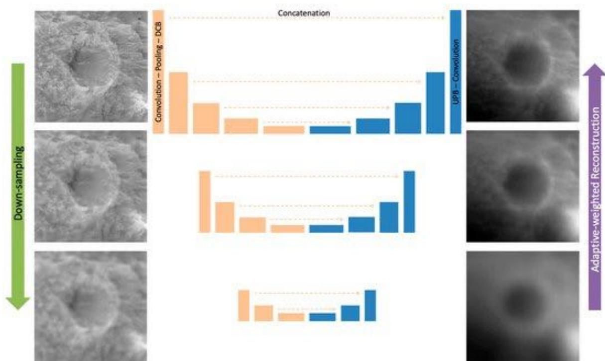
Figure 3. Overview of the MADNet generator network architecture. The input image has a size of  $512 \times 512$  pixels and the final output height map has a size of  $256 \times 256$  pixels in a relative value range of  $(0, 1)$ .
