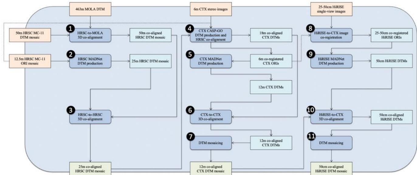
*Figure 4. Overall processing chain of the large area multi-resolution (HRSC-CTX-HiRISE) 3D mapping work. Inputs are shown with the light orange boxes, intermediate products with the light blue boxes, and final outputs are shown with the light green boxes.*
