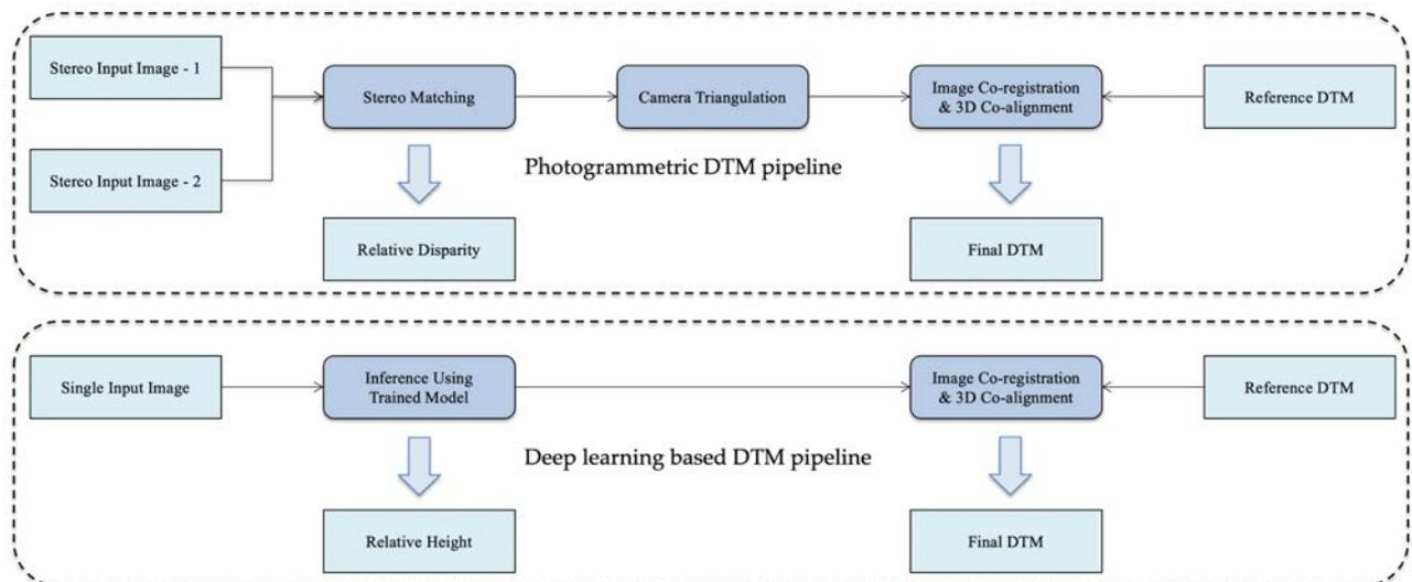
Figure 1. Illustration of the major differences between the photogrammetric DTM pipeline and the deep learning-based single-image DTM pipeline (e.g., MADNet) discussed here. Taken from (*Tao et al., RS, 2021d*).
