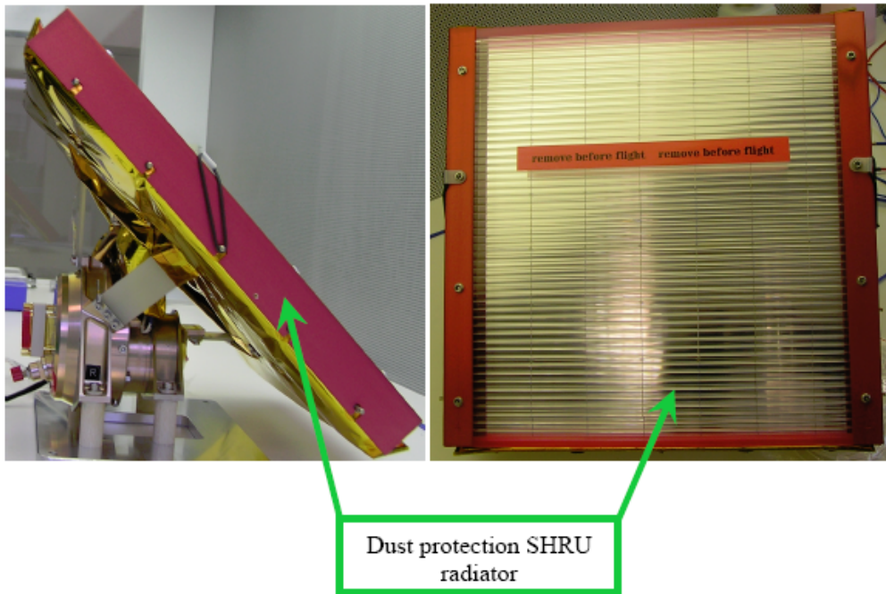
Figure 28 SHRU radiator dust protection.
