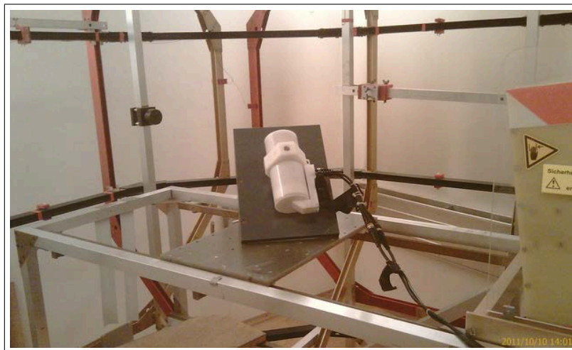
Figure 6: Overhauser Magnetometer Sensor in Diagonal in Space Orientation, CoC, View from South-West
