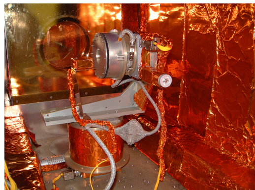
Figure 3: The Venus Express ASPERA-4 ELS sensor mounted in the MSSL calibration facility
