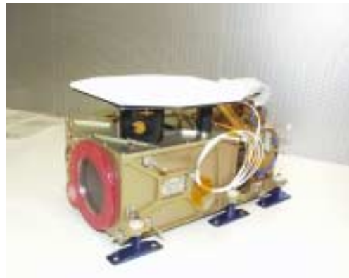
Figure 5 a/b: The SIR Instrument Unit from different viewing geometries. The O-Box is located in the front (right image, below white radiator). The dust cap of the aperture (red) is visible too. The sensor-head (spectrometer) is located behind the optical box (right image) and connected with a cooling band (white) to the radiator. A special fiber-optics (silver cable in left image) connects the focal plane of the off-axis mirror system with the interior of the sensor-head. The isostatic mount consists of five feet (blue).
