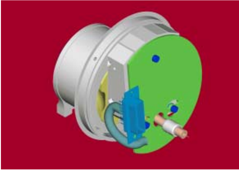
Figure 8: Drawing of the integrated sensor-head with removed cap. The electrical connector J4 (blue) and the mounting pins (blue) of the PCB (green) are visible. Quartz housing and cooling finger are made from aluminum (silver). A small part of the quartz body is also visible (gold-yellow). The optical fiber (pink) pierces the PCB.
