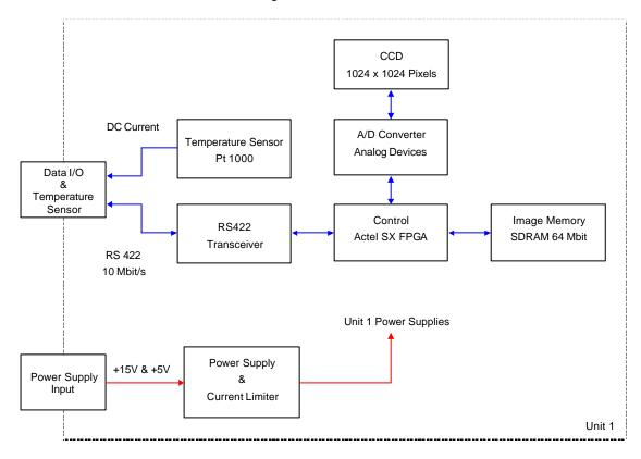
Figure 5: Unit 1 Electrical Design Description
