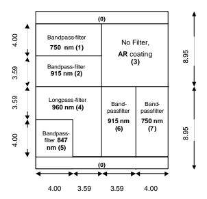
Figure 6: Filters in front of the CCD
