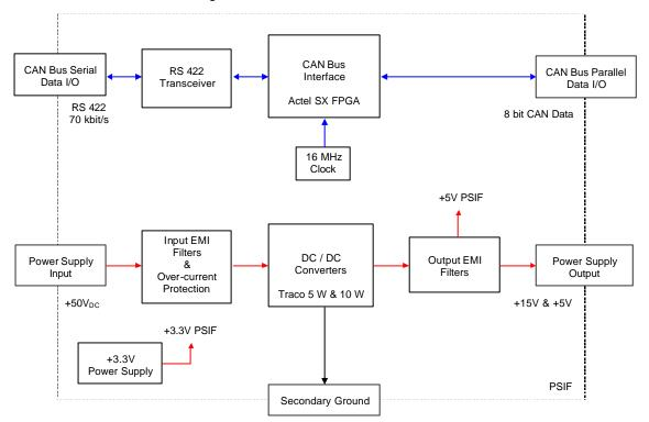
Figure 11: Electrical Design Description of PSIF Board
