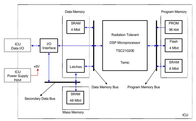
Figure 17: Electrical Design Description of Image Compression Unit Cube
