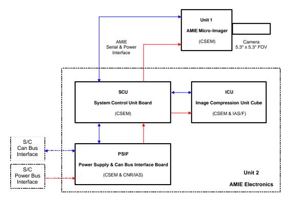
Figure 2: AMIE Imaging System - Main Hardware Functions
