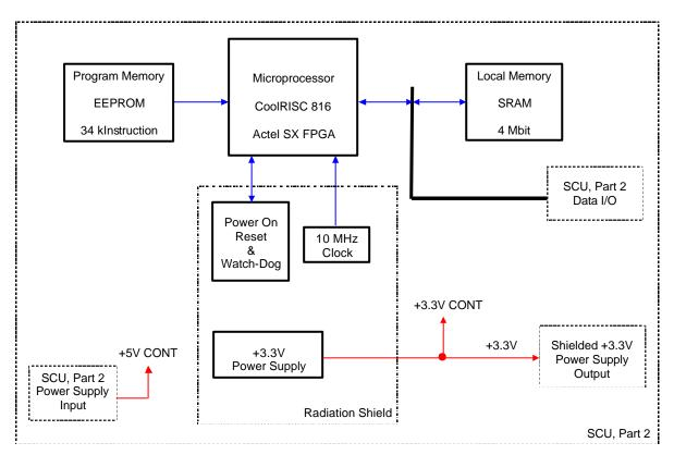
Figure 15: Electrical Design Description of SCU Board System management
