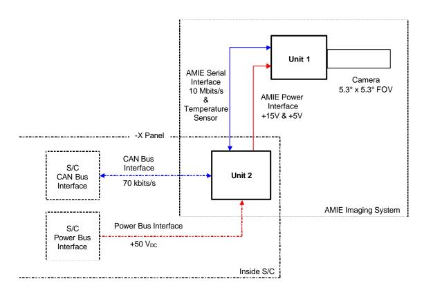
Figure 1: AMIE Imaging System - I/O Diagram
