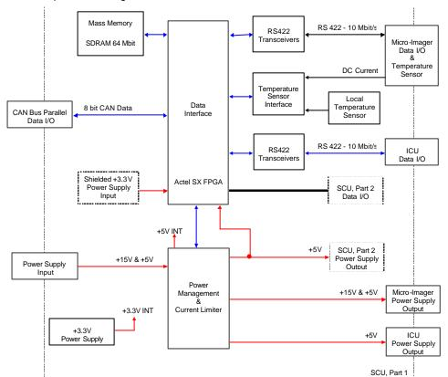
Figure 14: Electrical Design Description of SCU - Data Interface & Power Management
