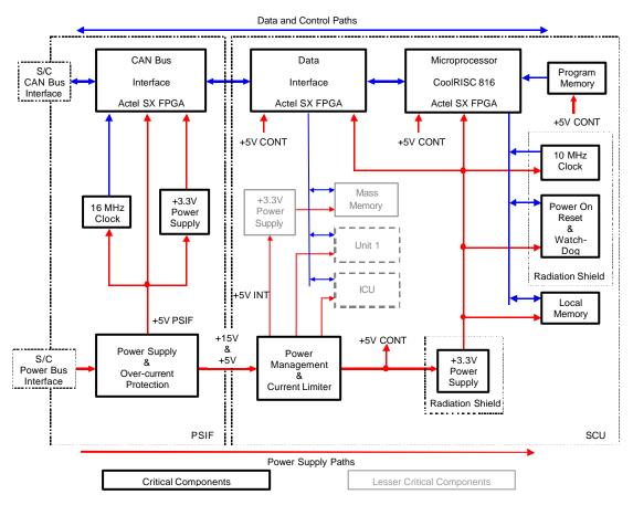
Figure 18: Radiation Tolerance Strategy with Respect to Analysis of Possible Failures
