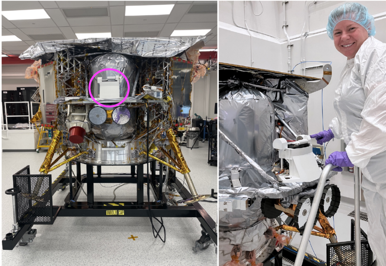
Figure 2. PITMS mounted to the Peregrine lander Deck D (left, magenta circle) in the Astrobotic cleanroom and (right) during remove-before-flight activities (with BAC for scale). The Iris rover [Potter, 2023] is mounted to the underside of deck D. The PITMS aperture opens to the +X direction of the spacecraft.
