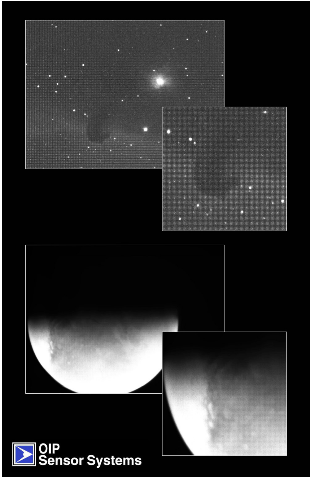
Figure 1: TIFF Bayer images of the Horse Head Nebula (crop of the original image) photographed with a Canon 20Da dSLR and Mars photographed with Mars Express' VMC camera. The enlarged images show clearly the Bayer pattern of the imaging sensor (visible as a grid).
