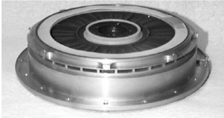
Figure 1.2.1 – The low energy neutral particle imager for the ASPERA-C/Mars-96 experiment (spare unit)
