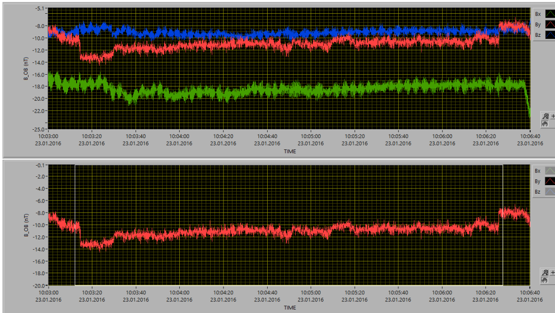
Figure 1: Examples of a WOL disturbance recorded on 23.01.2016 during the EXT1 phase with the OB sensor. Top: The x-axis shows time, the y-axis shows all three magnetic field components. Bottom: y-component of the magnetic field. The white box marks the duration of the WOL disturbance.
