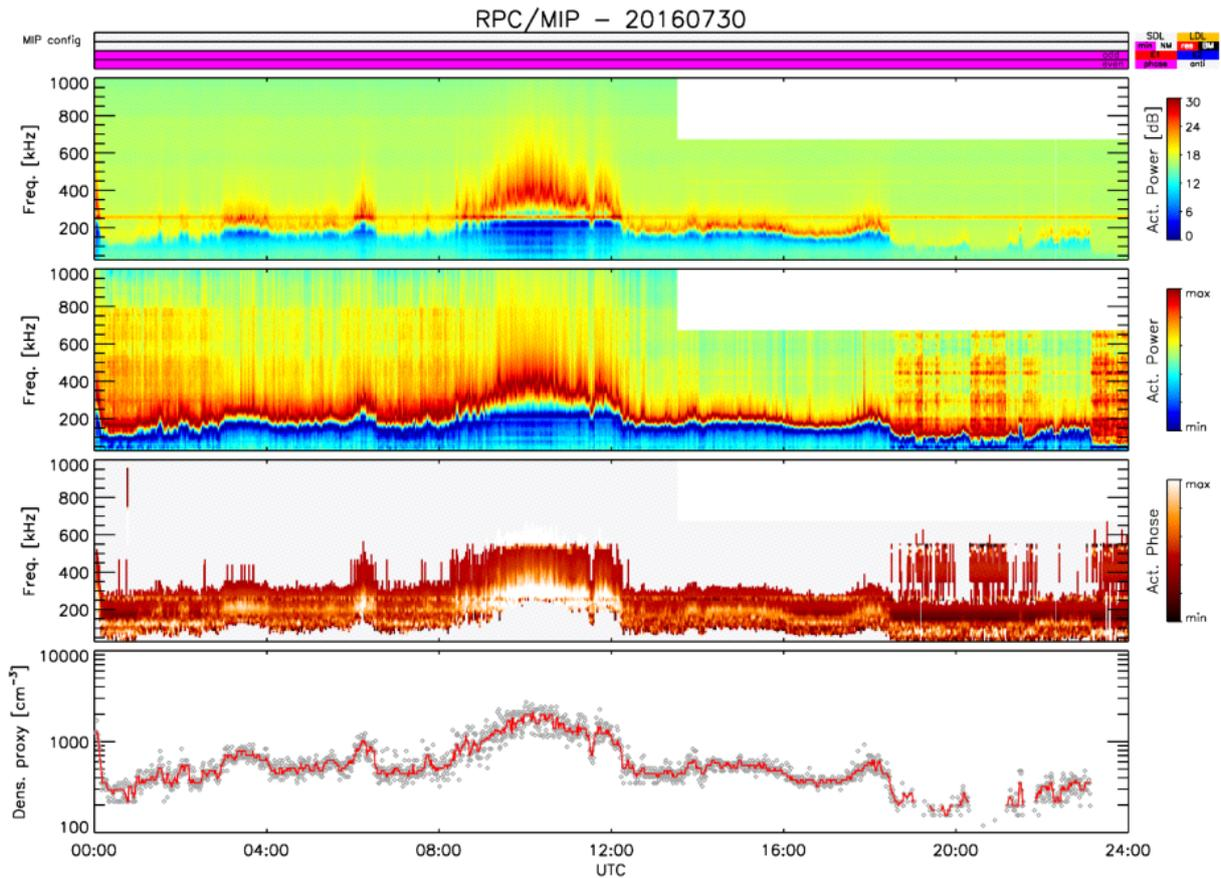
Figure 3.11: Example of RPC-MIP data overview during a full day in 30 July 2016, from top to bottom: (i) MIP operational parameters, (ii) calibrated active MIP power spectrogram (Level 3), (iii) rescaled calibrated active MIP power spectrogram (Level 3), (iv) rescaled calibrated active MIP phase spectrogram (Level 3), (v) retrieved MIP densities (grey dots) and moving averaged density (red line) (Level 5).
