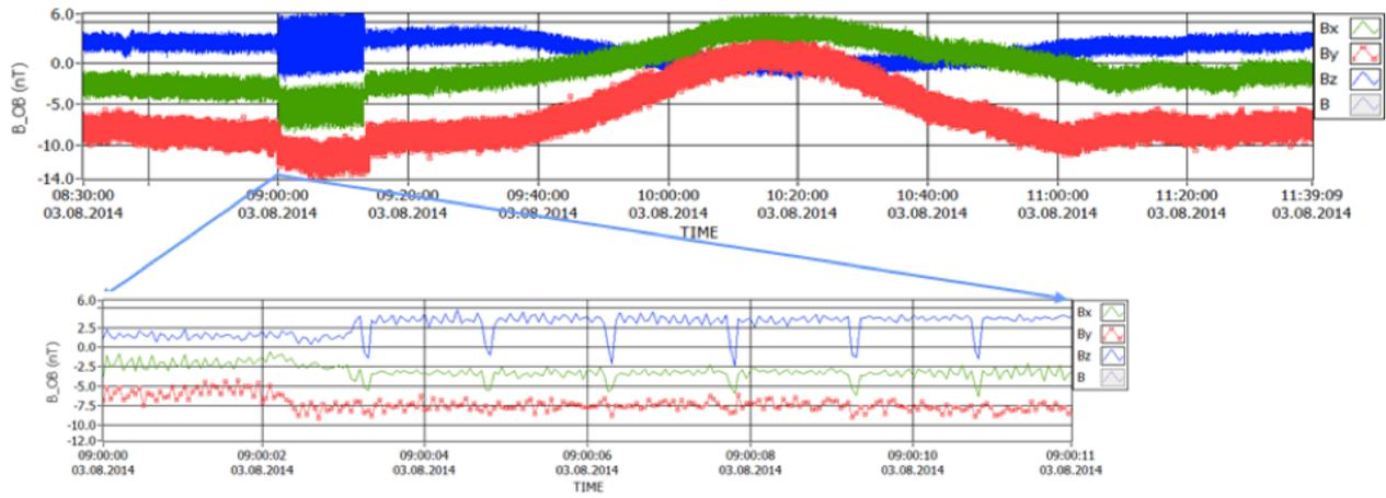
Figure 3.17: Disturbance by thruster activation during OCMs. Besides DC-jumps of  $\sim 2$  nT additional AC spikes of  $\sim 6$  nT spikes, at  $\sim 625$  mHz, and  $\sim 200$  ms width appear. An automatic cleaning of these structures is hardly possible, but the data in these intervals will be flagged as bad data in the final datasets.
