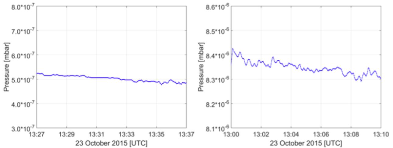
Figure 3.23: From Tzou (2017). Example of measurements by COPS with (left) and without (right) plasma in the chamber. Plasma inside the chamber makes COPS measurements less reliable: the pressure measured is higher, spikier and variable on short timescales.
