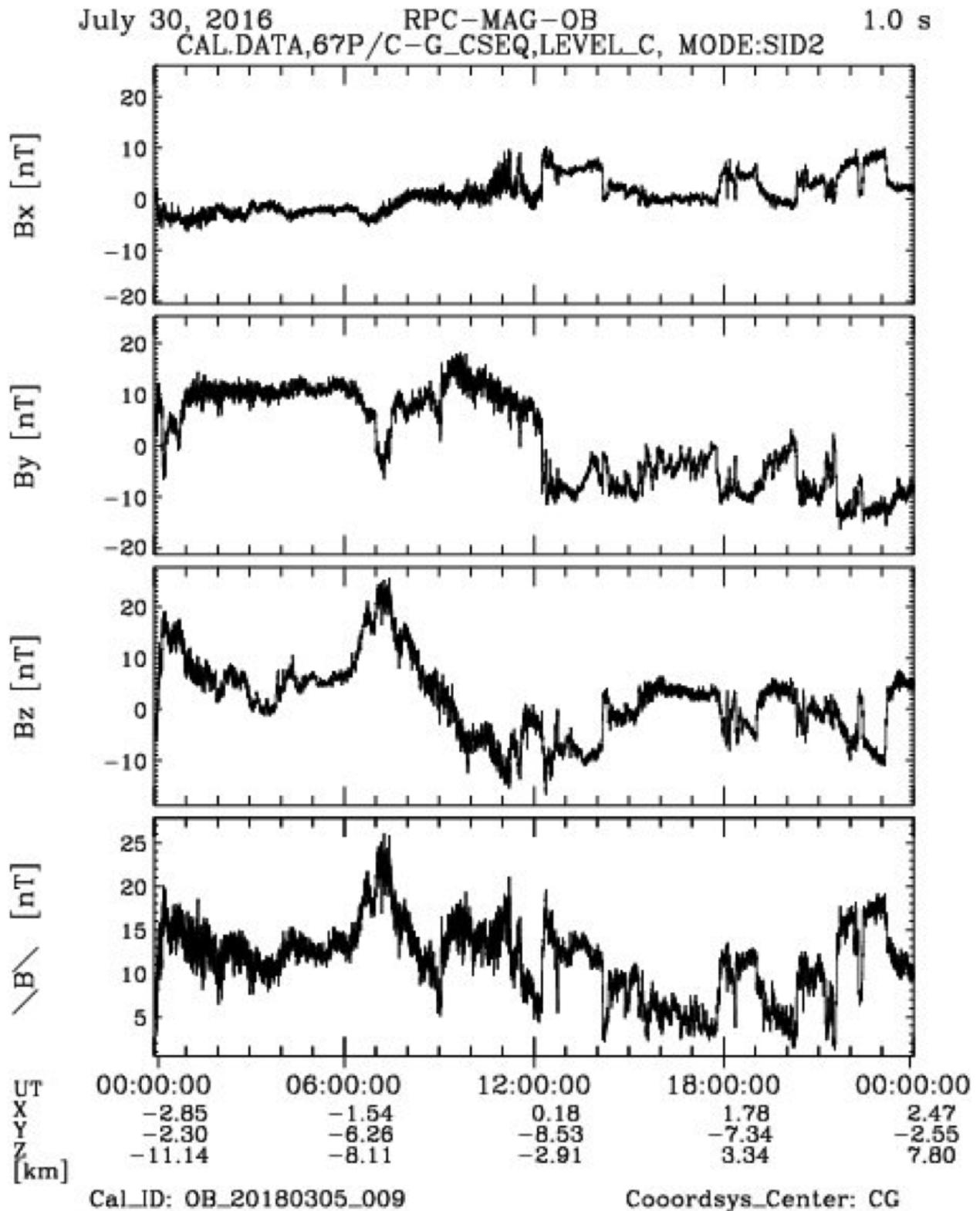
Figure 3.12: Overview of the three magnetic field components and magnetic field magnitude on July 30<sup>th</sup>, 2016. The data is shown in the CSEQ reference frame with highest available resolution (Level C, L3) data resampled to 1 Hz. Auxiliary data is given at the bottom.
