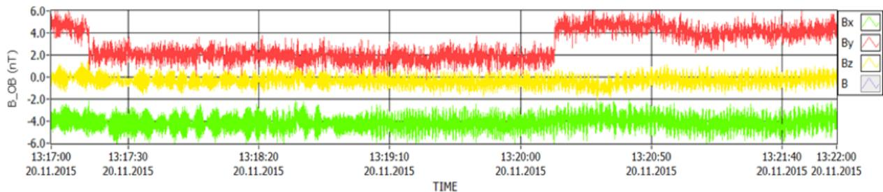
Figure 3.16: Disturbance by thruster activation during WoLs on LEVEL\_C (L3) magnetic data. A clear shift of the spacecraft residual field in the order of  $\sim 3$  nT can be seen while the latch valves of the thrusters are activated. The WoL activation is deterministic and known, thus these periods can be flagged as bad data.
