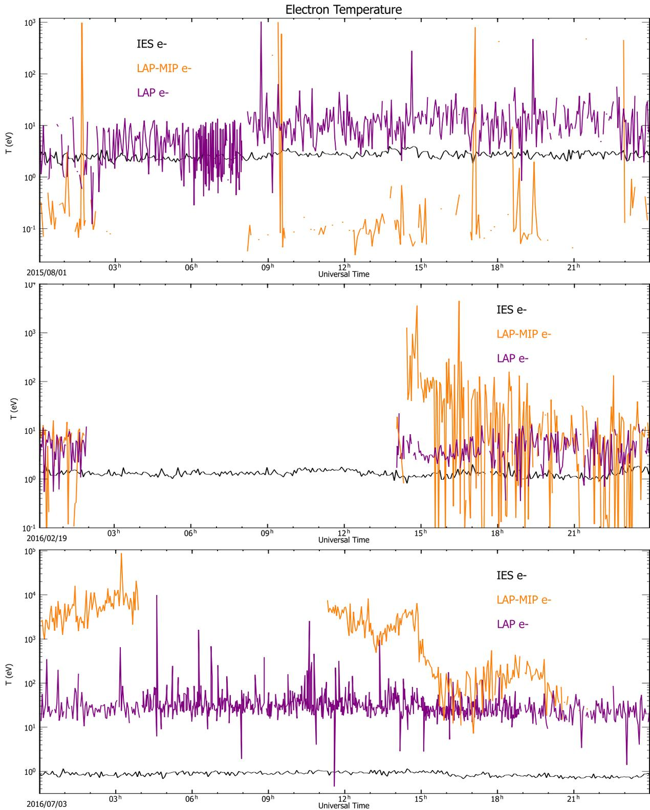
Figure 2.12: Electron temperature from RPC-IES, RPC-LAP and cross-calibration LAP-MIP the 1<sup>st</sup> of August 2015 (upper panel), the 19<sup>th</sup> of February 2016 (middle panel), and the 3<sup>rd</sup> of July 2016 (lower panel).
