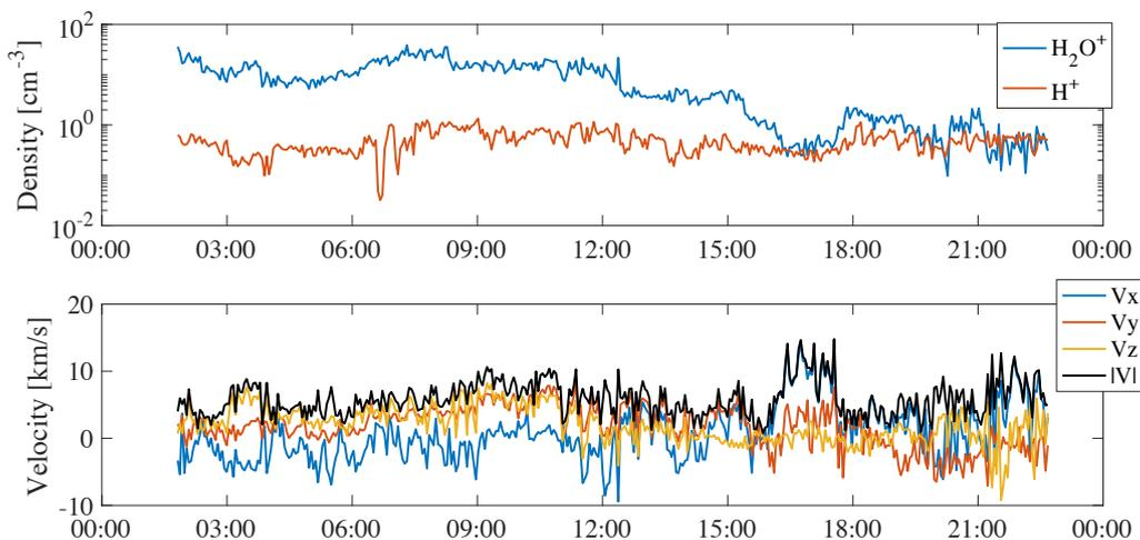
Figure 3.2: Upper panel: Number density (from Level 3) of the cometary ions (blue line) and of the solar wind ions (red line), obtained through integration of the observed fluxes [ $cm^{-3}$ ]. Lower panel: Bulk velocity (from Level 3) of the cometary ions [ $km \cdot s^{-1}$ ]. Note that these may be strongly affected by the spacecraft potential as well as restricted field of view.
