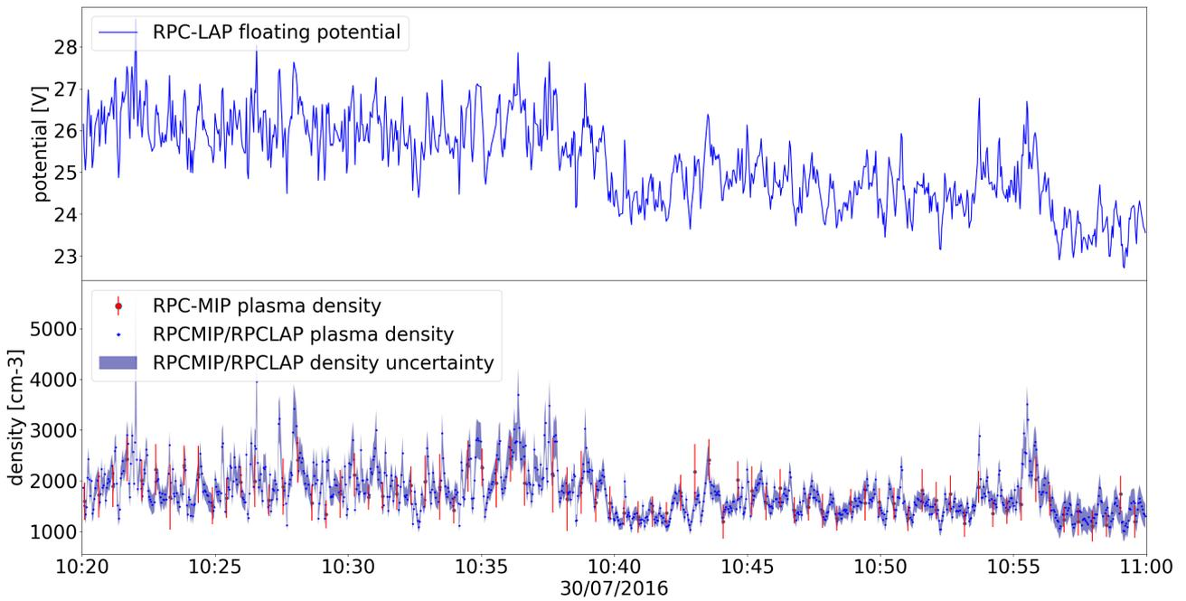
Figure 2.3: Example of RPCMIP/RPCLAP cross-calibrated densities over 20 minutes for 30 July 2016, from top to bottom: (i) RPC-LAP MIP floating potential used as input to the cross-calibration procedure, (ii) RPC-MIP plasma density (Level 3) used as input to the cross-calibration procedure and resulting RPCMIP/RPCLAP cross-calibrated plasma densities with associated uncertainties (Level 5).
