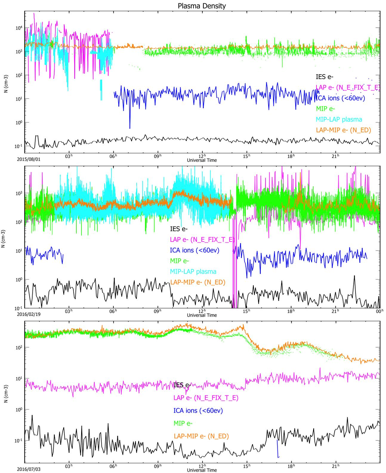
Figure 2.6: Plasma (electron or ion) number densities from RPC-MIP, RPC-LAP, RPC-ICA, RPC-IES and cross-calibrations between MIP and LAP the 1<sup>st</sup> of August 2015 (upper panel), the 19<sup>th</sup> of February 2016 (middle panel), and the 3<sup>rd</sup> of July 2016 (bottom panel). The ion number density from RPC-ICA has been derived from ions at energies between a few eVs (not 0) and 60 eV.
