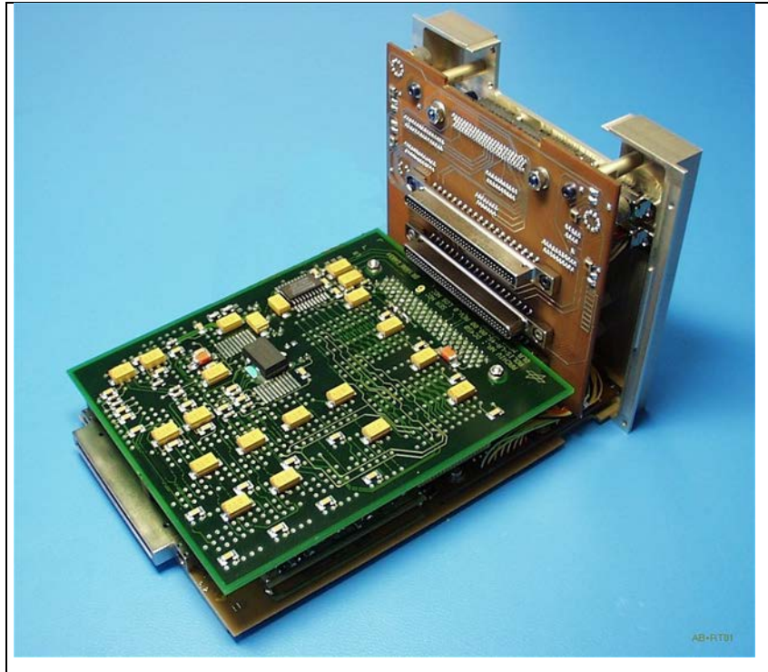
Figure 6.6-3: IME BackPlane [IME 2-04F] before integration into PIF [IME 2-00F]
